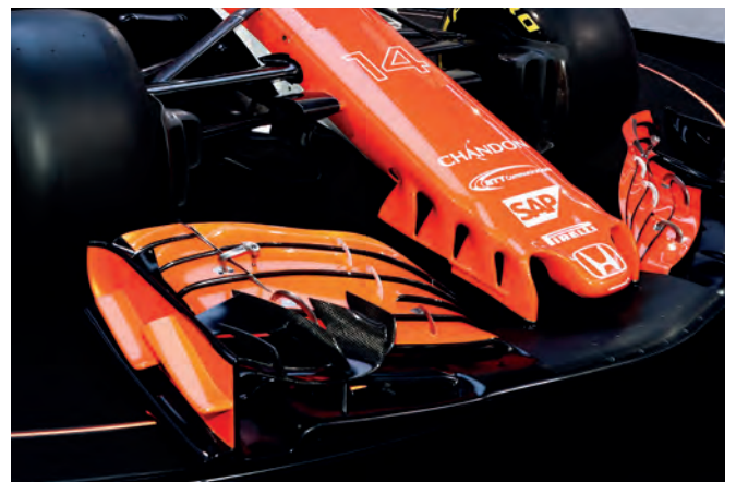
Figure 2: Front wing design of Formula One cars from 1988 and 2017. The greater understanding of the cars' aerodynamics has allowed for more intricate geometrical designs to achieve greater performance. McLaren Racing
