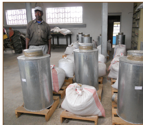
Metal Storage Silo —adapted for smaller capacity for use by smallholder farmer
