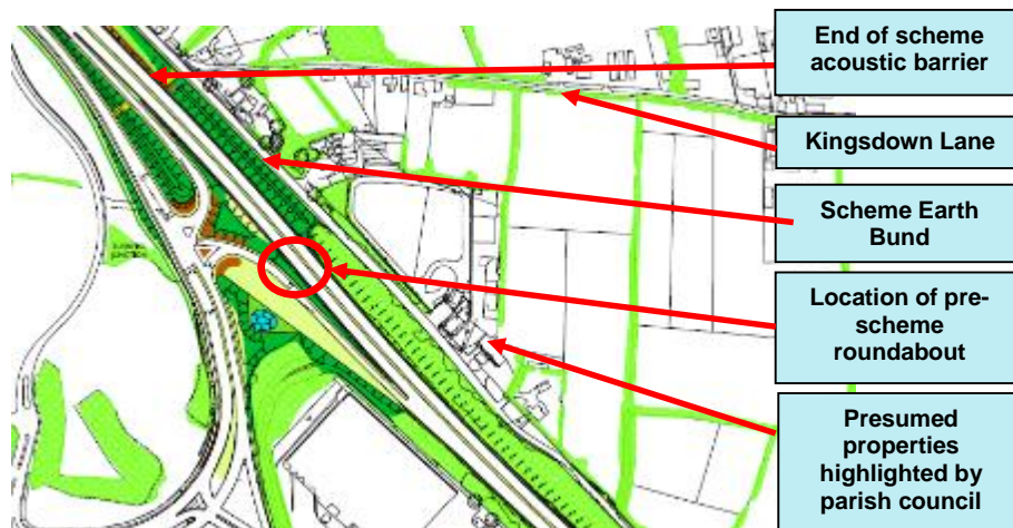
Figure 5.2 – Environmental Design Drawing (south) figure 5.0b with annotations showing installed features and the original location of Turnpike Roundabout
