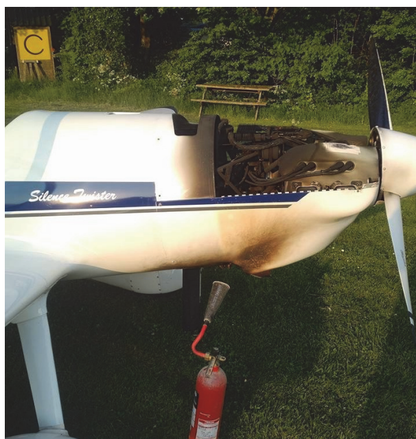
Figure 1 G-TWSS after the fire was extinguished
