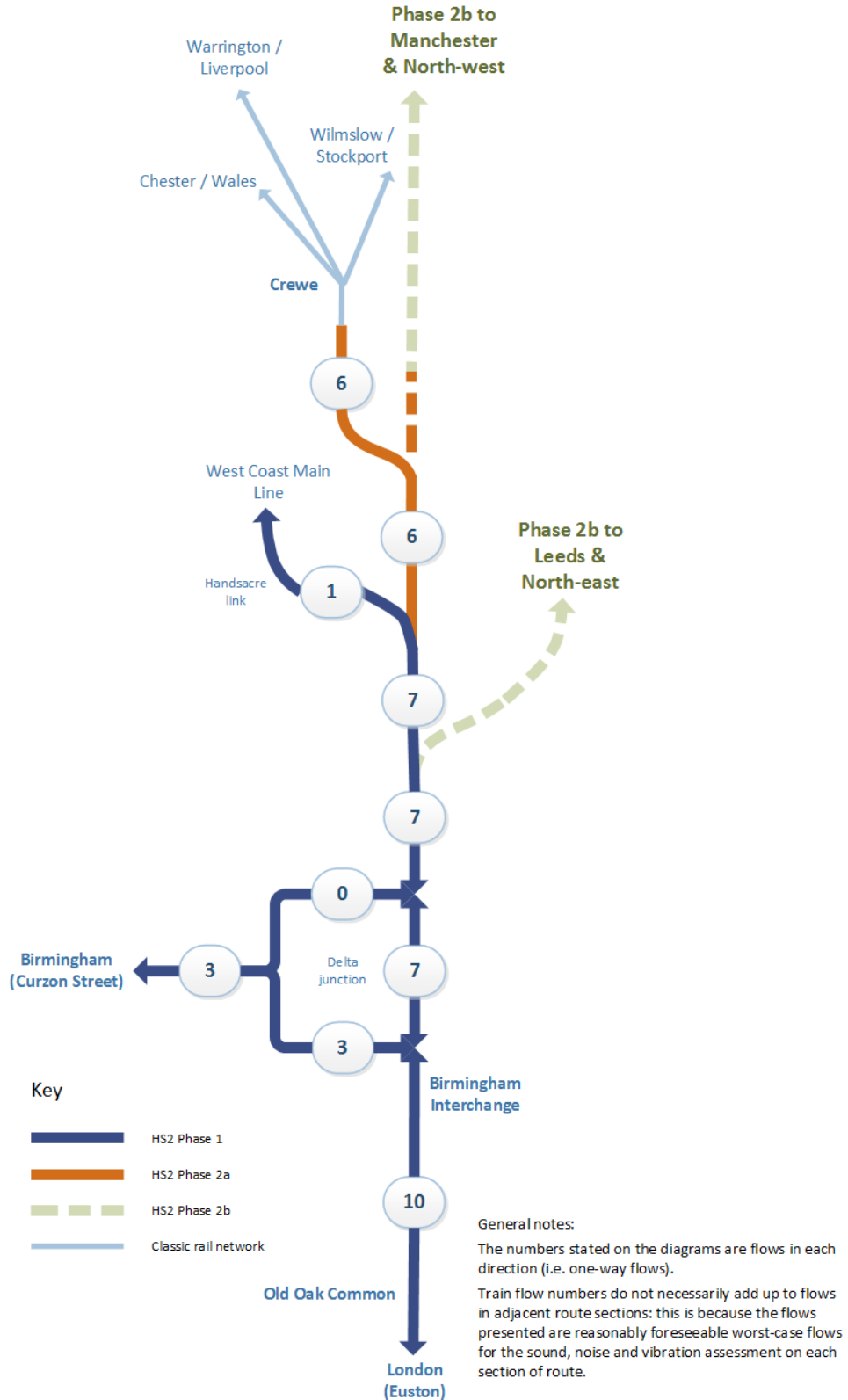
Figure 4: Proposed Scheme – peak hour one-way train flow (Phase 2a year of opening 2027)
