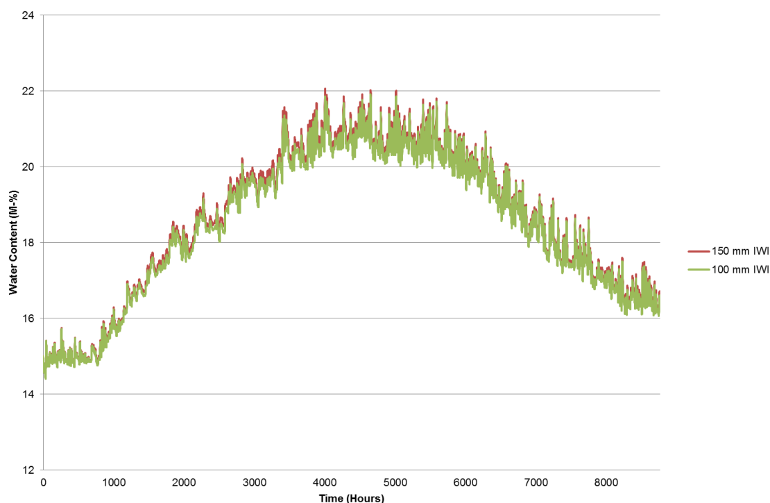
Figure 6-12 Water Content (M-%) End of Perpendicular Intermediate Floor Joist
