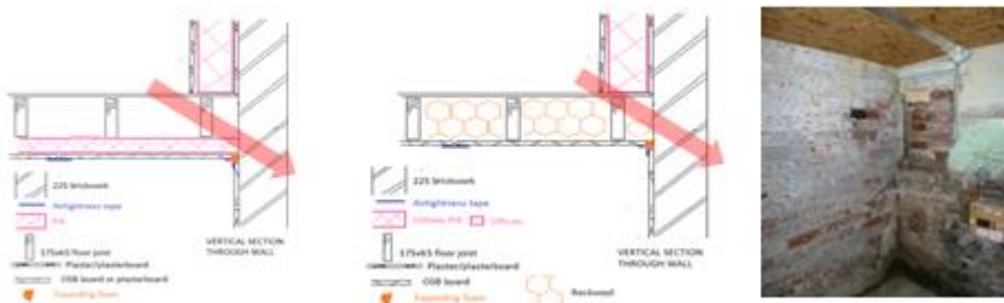
Figure 2-9 Ground floor wall junction, especially typical at pre-1919 properties with basements. Some holes into floor voids are not taped/sealed. Where the floor between the basement and ground floor is not fully and carefully insulated, thermal bridges can occur
