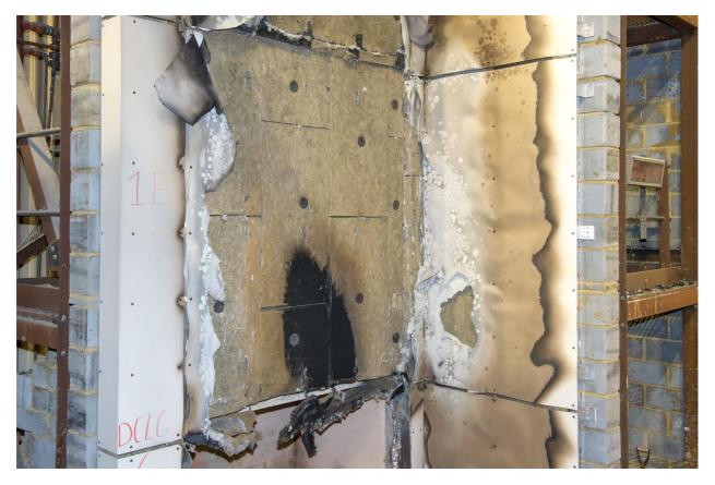
Figure 20. First row ACM panels (directly above combustion chamber).
