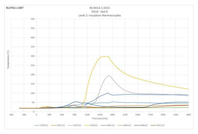
Figure 18. Level 2 insulation thermocouples.
