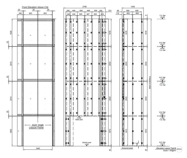
Figure 11. Front elevation, side elevation and vertical sections for the substructure system (supplied by the Test Sponsor).
