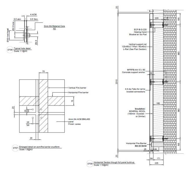
Figure 14. Vertical section through the cladding system, ACM panel detail and vertical and horizontal fire barriers intersection (supplied by the Test Sponsor).
