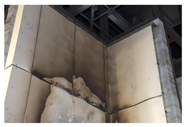
Figure 22. Third row ACM panels (approximately 4600mm-6500mm above combustion chamber).
