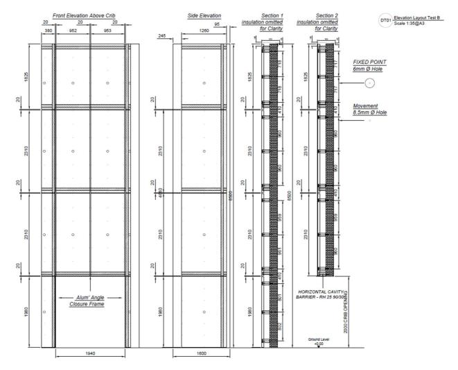
Figure 10. Front elevation, side elevation and vertical sections for the system (supplied by the Test Sponsor).
