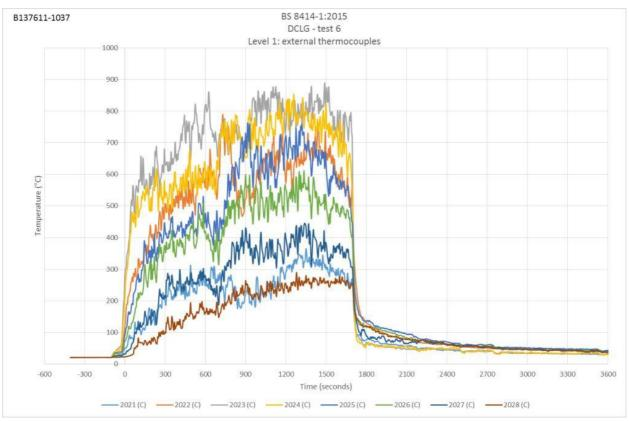
Figure 15. Level 1 external thermocouples.  $t_s$ =105s after ignition of the crib.
