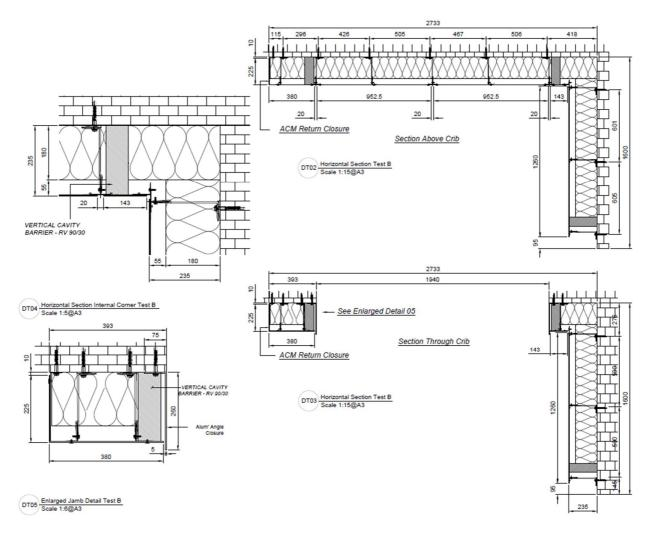
Figure 13. Horizontal section through and above the combustion chamber, and installation details for the system (supplied by the Test Sponsor).
