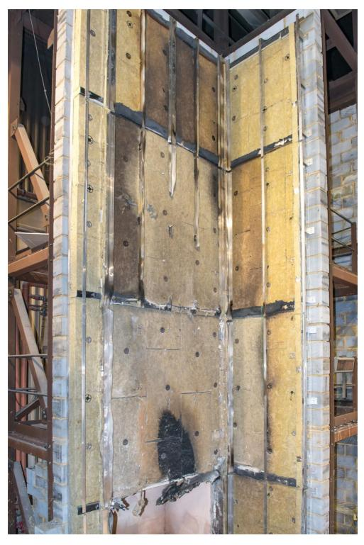
Figure 25. Full height photograph of cladding system following removal of ACM panels.
