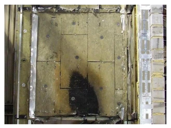
Figure 24. Close up of charred section of stone wool insulation directly above the combustion chamber.
