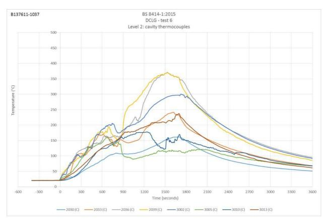
Figure 17. Level 2 cavity thermocouples.  $t_s$ =105s after ignition of the crib.
