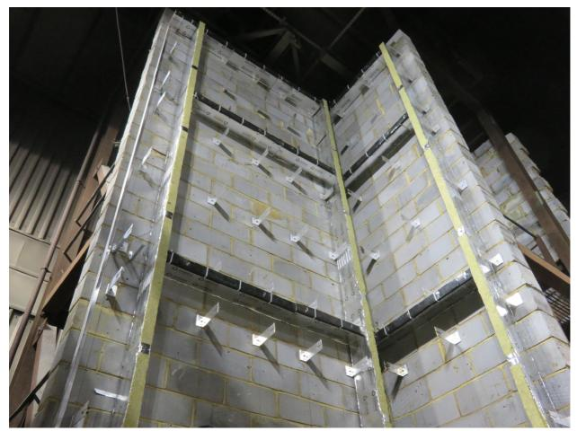
Figure 3. Location of 'L' brackets and cavity barriers.
