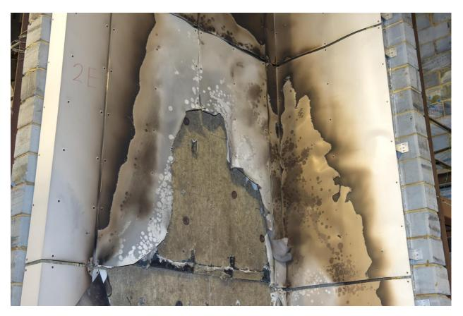
Figure 21. Second row ACM panels (approximately 2300mm-4600mm above combustion chamber).
