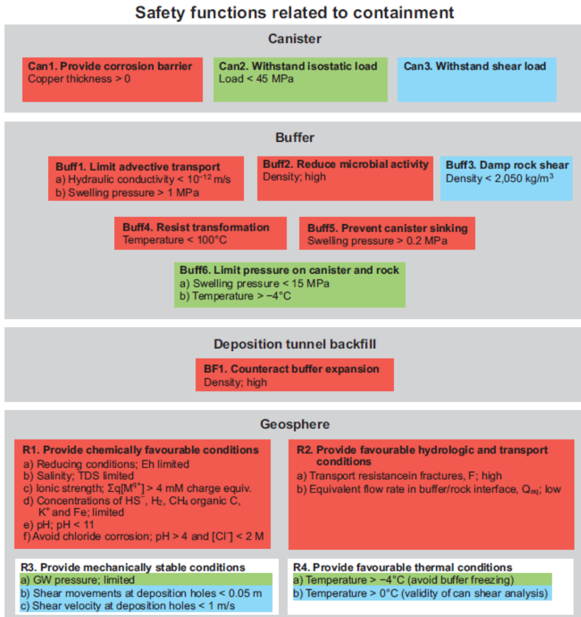
Figure 3.9 Safety functions, safety function indicators and safety function indicator criteria related to containment
