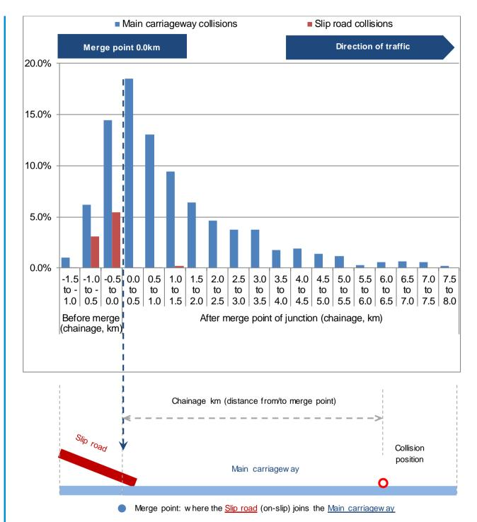
Figure 5-35 Combined distribution of collisions from respective merge points
