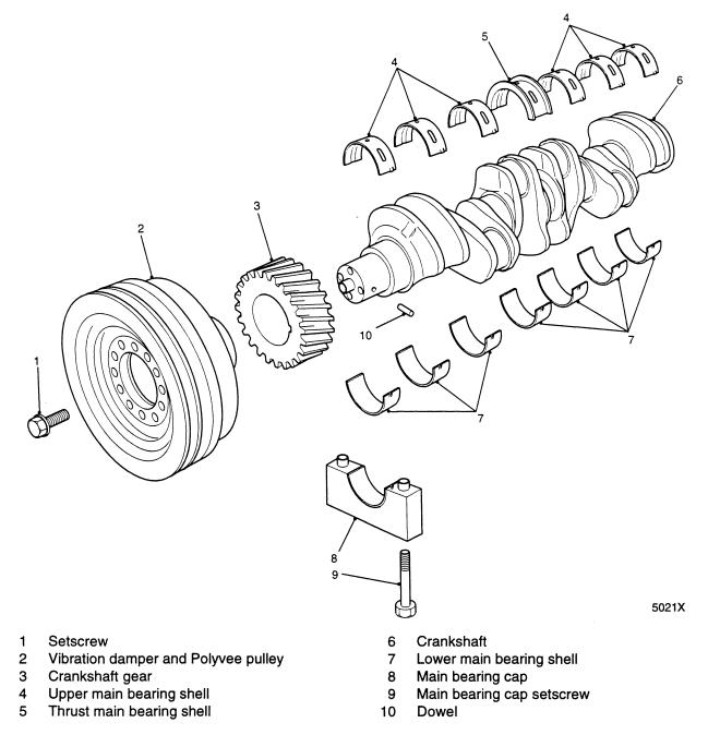
Fig 4 Crankshaft assembly
