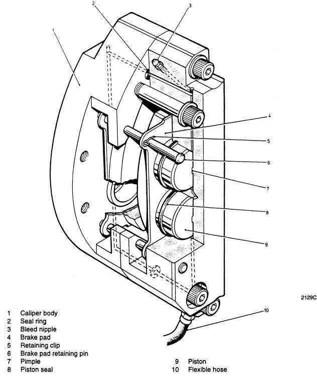
Fig 7 Main brake caliper
