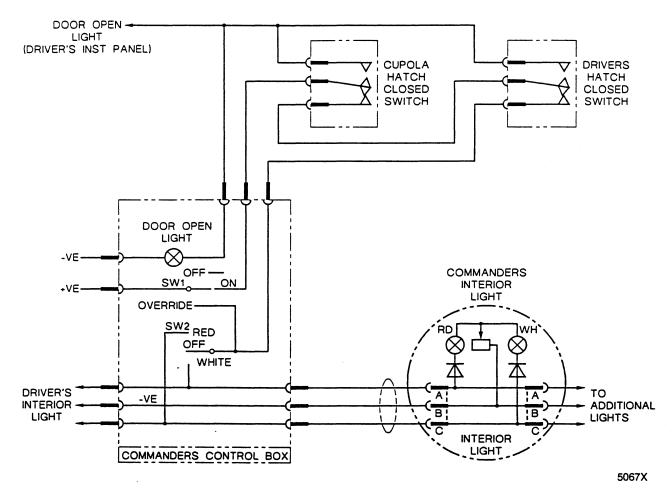
Fig 10 Interior lighting - schematic
