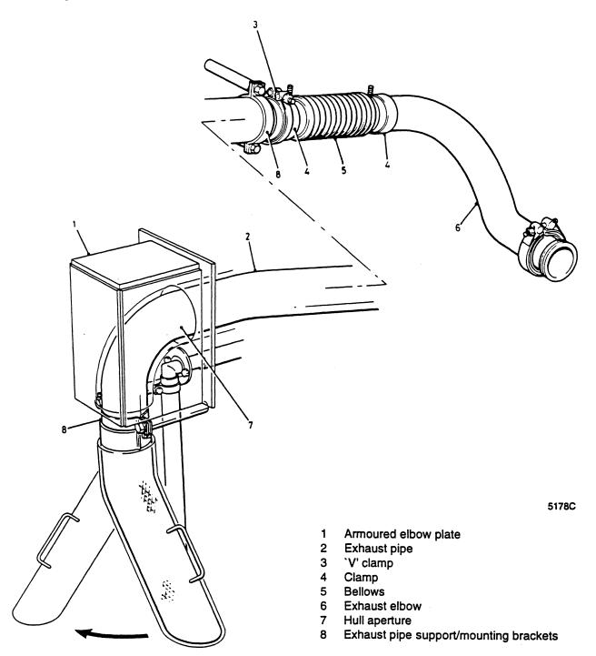
Fig 7 Exhaust pipe and fittings
