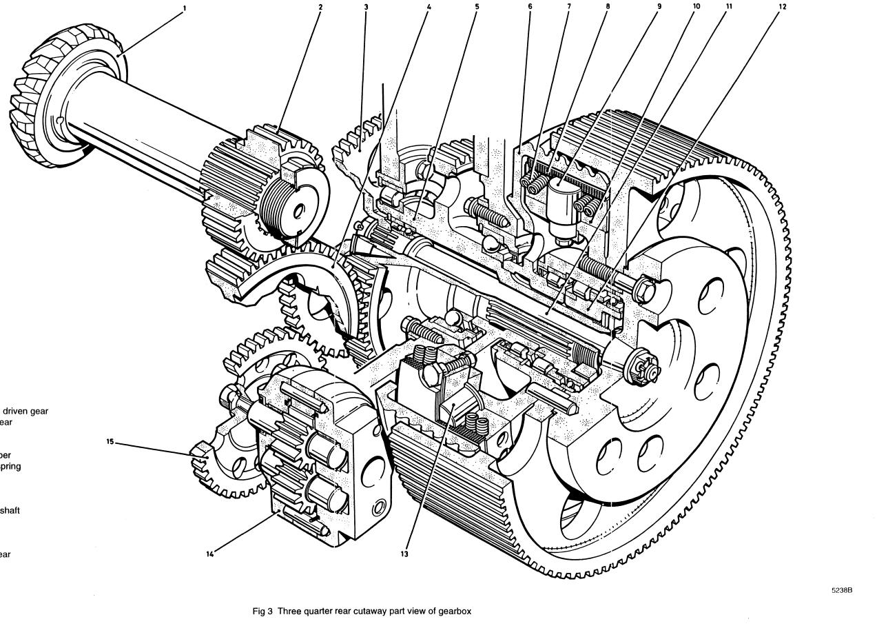
Fig 3 Three quarter rear cutaway part view of gearbox
