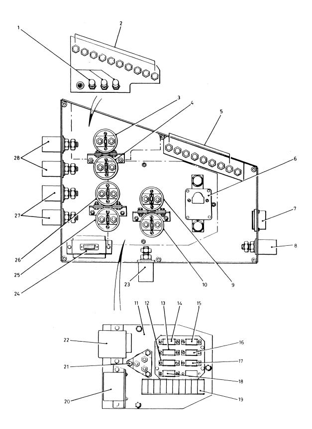
Fig 4 Distribution panel - internal layout
