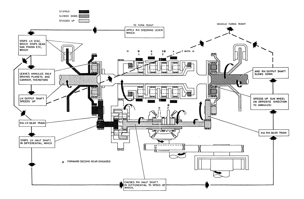
Fig 7 Steering operation - gearbox
