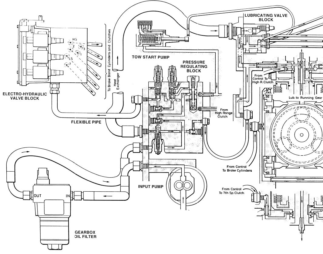
Fig 10 Hydraulic and lubricating system
