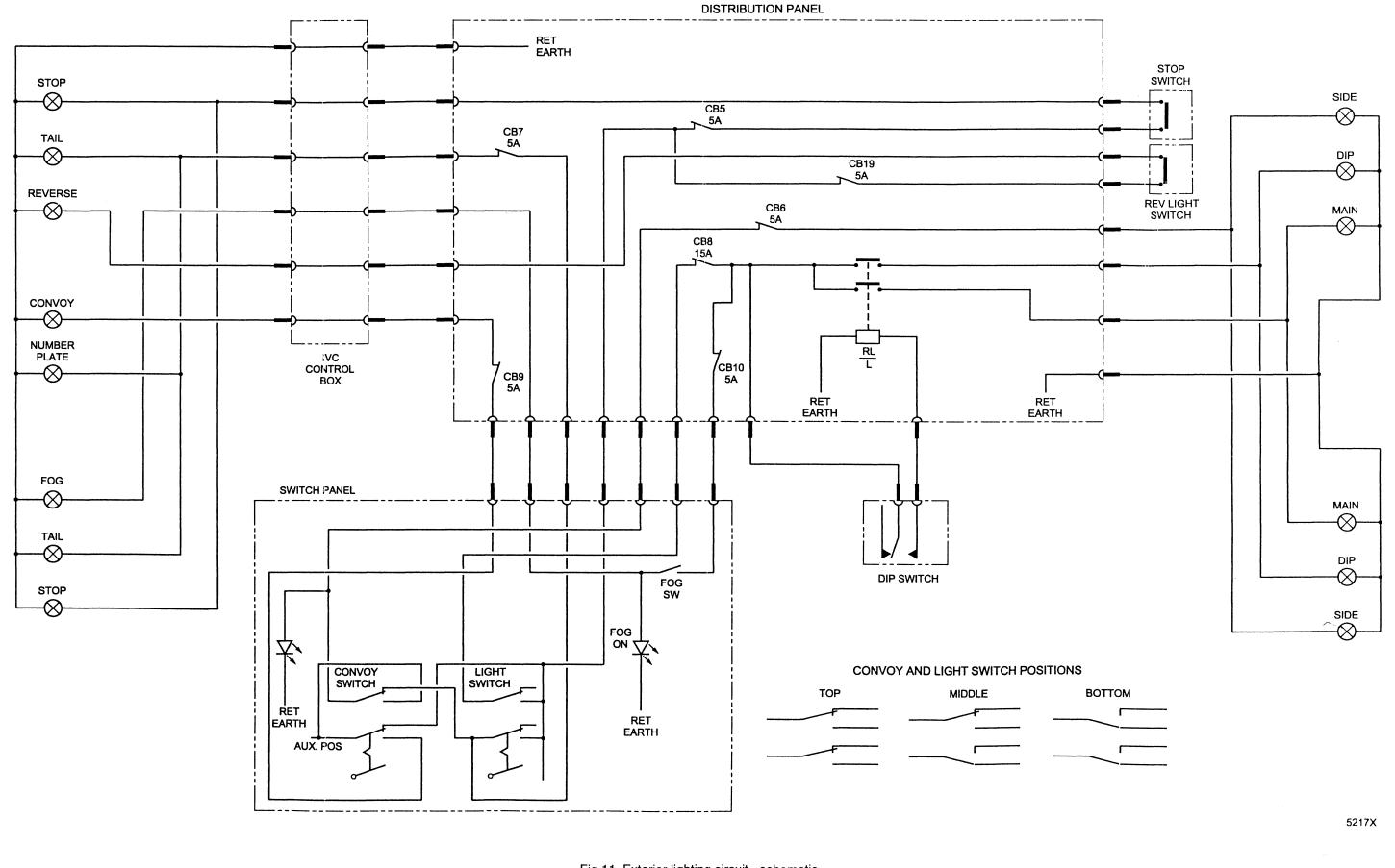
Fig 11 Exterior lighting circuit - schematic
