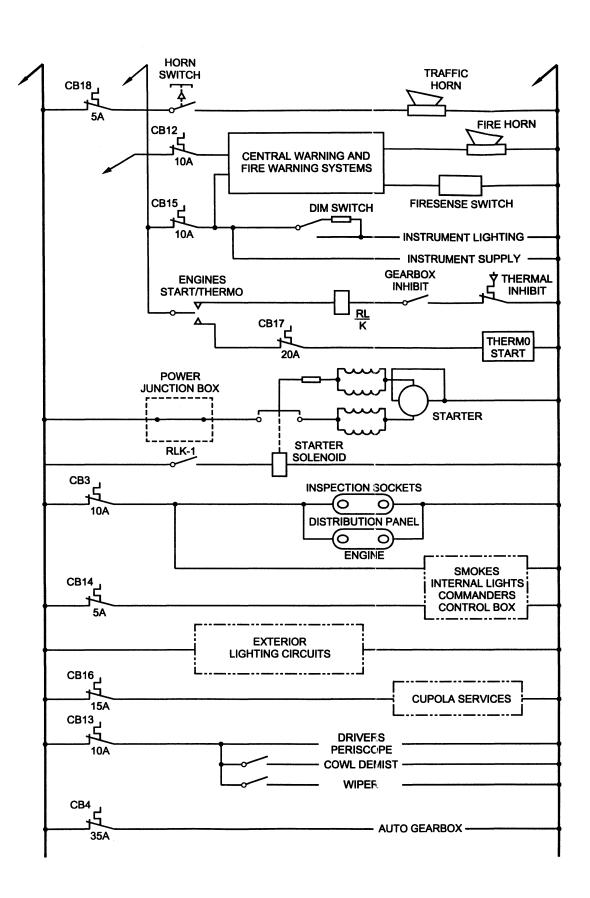
Fig 3 Distribution panel circuit - schematic
