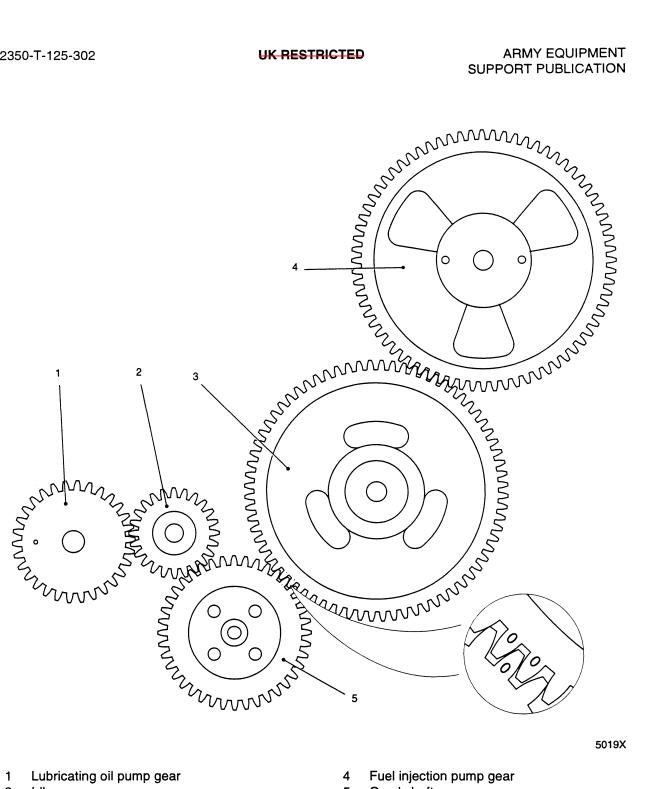
Lubricating oil pump gear 1
