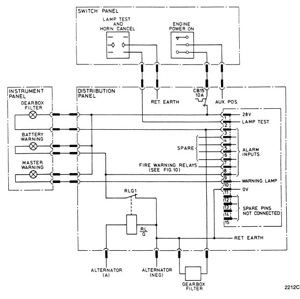
Fig 8 Central warning system - schematic
