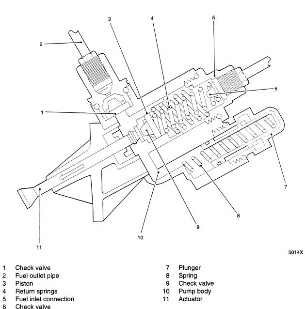
Fig 6 Fuel lift pump
