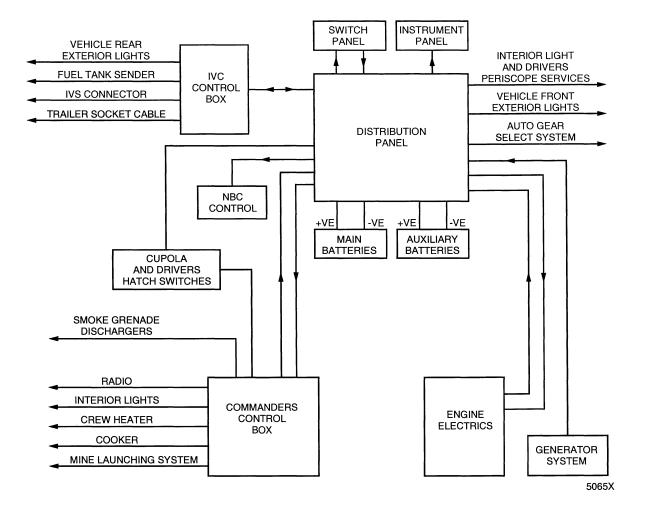
Fig 1 Vehicle electrical system - schematic
