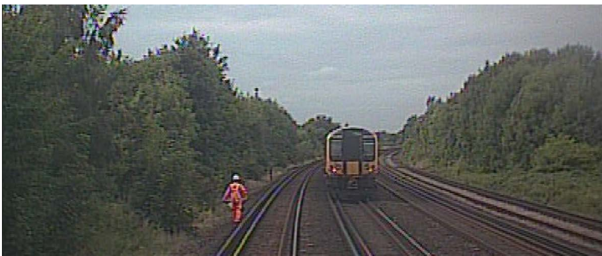
Forward facing CCTV image from the train that struck the track worker, looking towards Raynes Park, showing the rear of the first train having passed the distant lookout (courtesy of South Western Railway)
