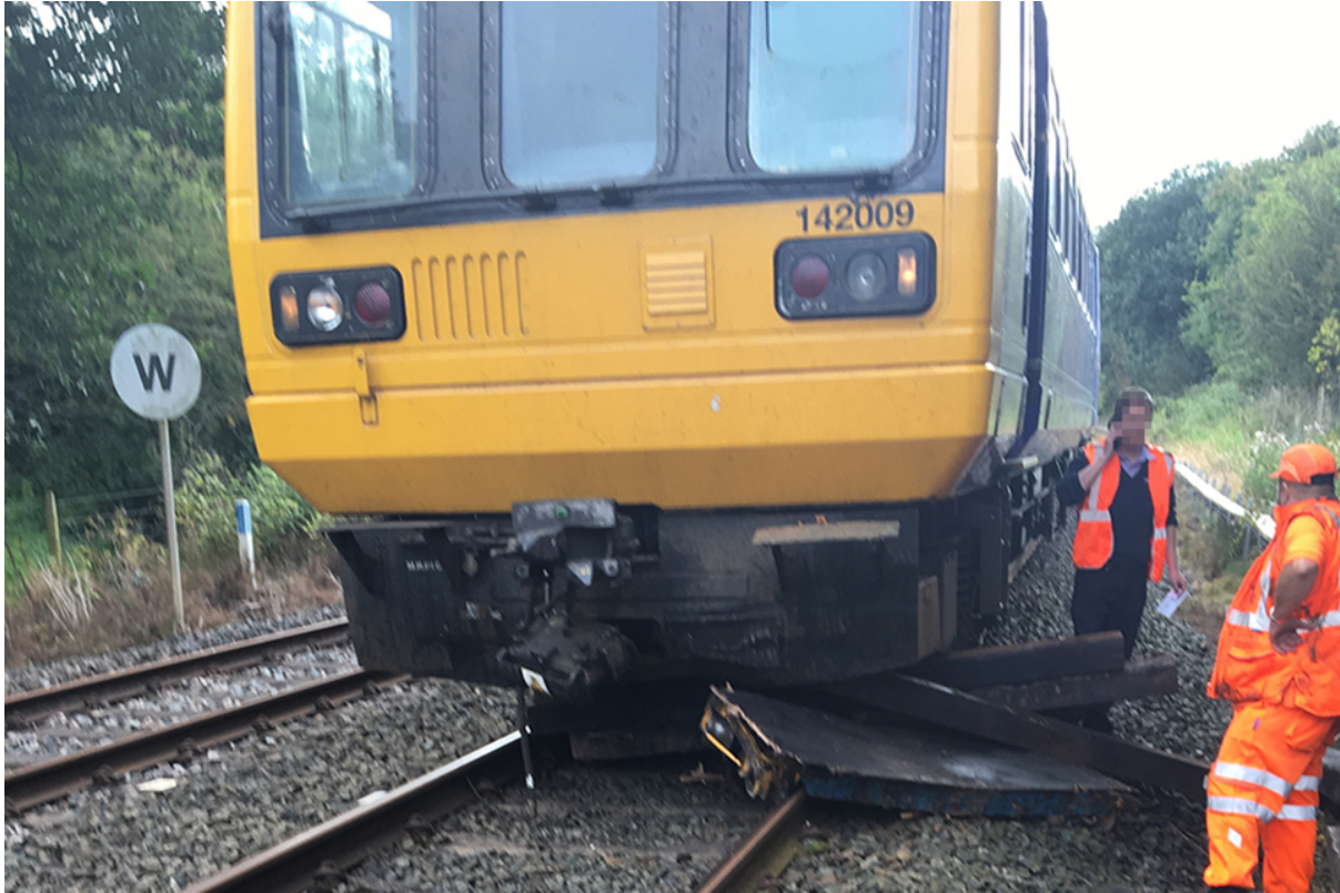
View of the front of train after collision with the trolleys
