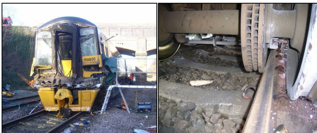
Figure 5: Derailment at Barrow on Soar; damaged leading end of train (left); guidance provided by the brake discs (right)
