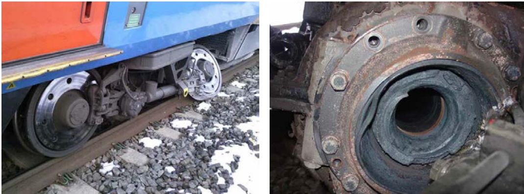
Figure 3: Passenger train derailment at East Langton; the derailed wheel (left) and the fractured axle (right)
