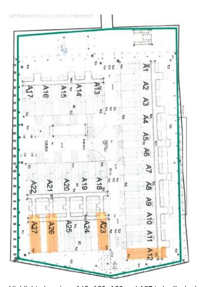
Highlighted engines A12, A23, A26 and A27 to be "locked out" so that only the other 23 engines may operate.
