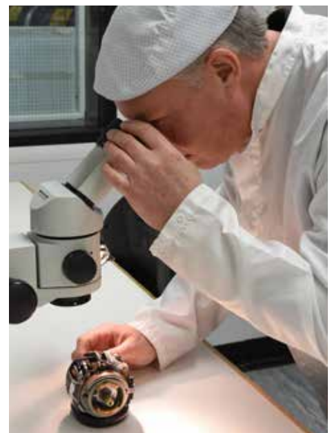
Inspection of the gimbal assembly from a vertical gyro that forms part of the automatic flight control system fitted to Lynx and Chinook helicopters
