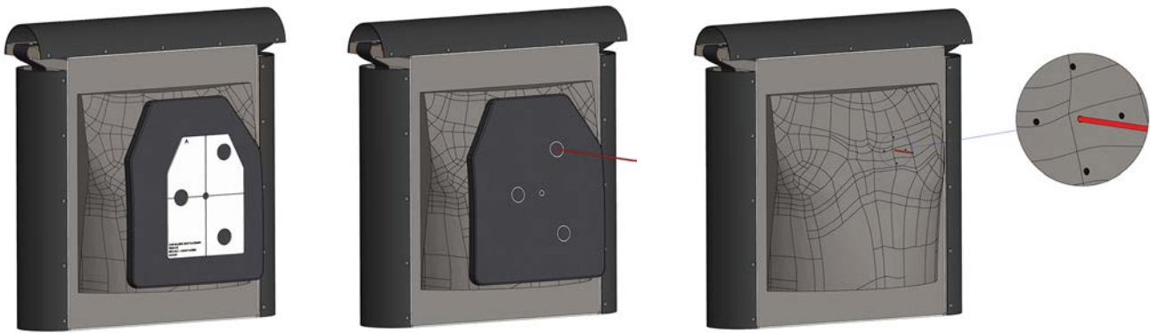
Figure 18: Marking of shot locations and measurement of pre-shot surface positions
