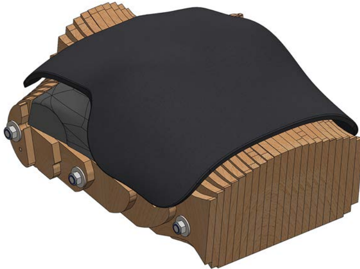
Figure 31: Formed armour stab test configuration
