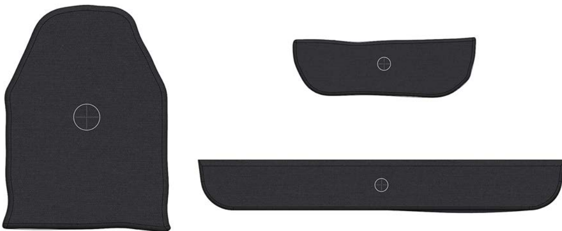
Figure 20: Example shot marking on extended coverage panels
