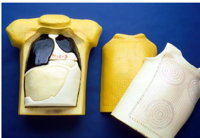
Figure 6 The Lawrence Livermore torso phantom used for Am-241 in lung calibrations
