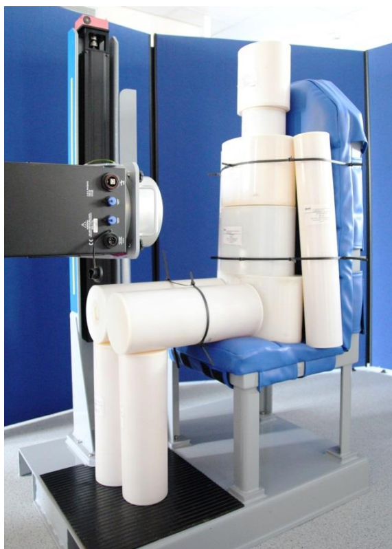
Figure 1 Transportable monitoring system in whole body measurement geometry showing BOMAB phantom
