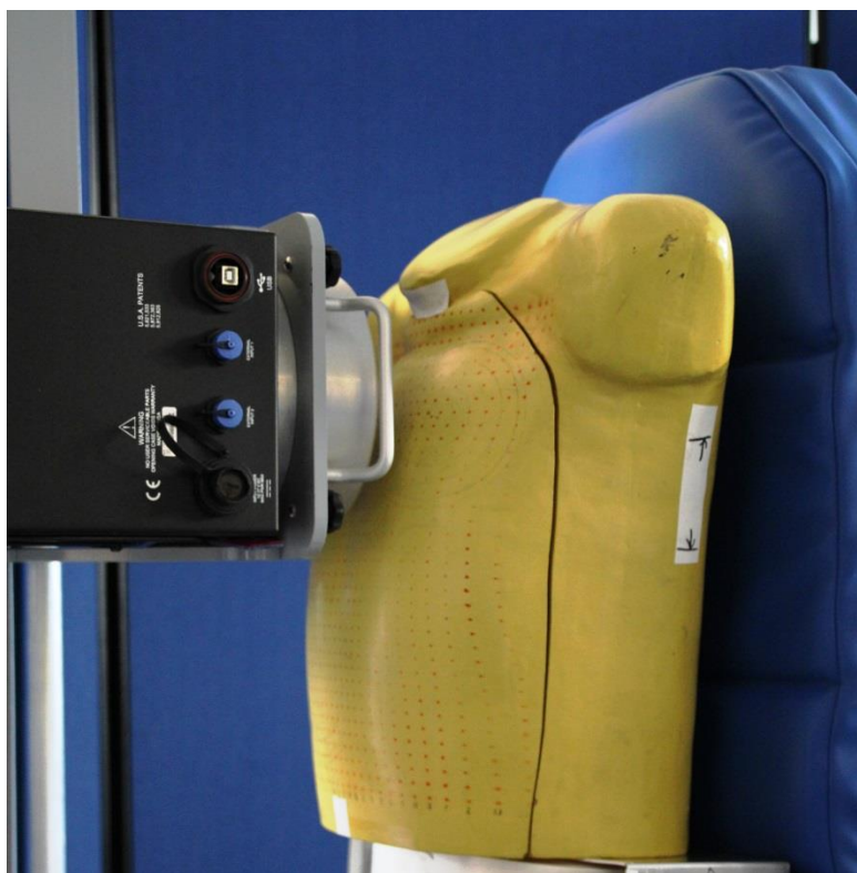
Figure 7 Lung counting geometry shown with Lawrence Livermore Phantom
