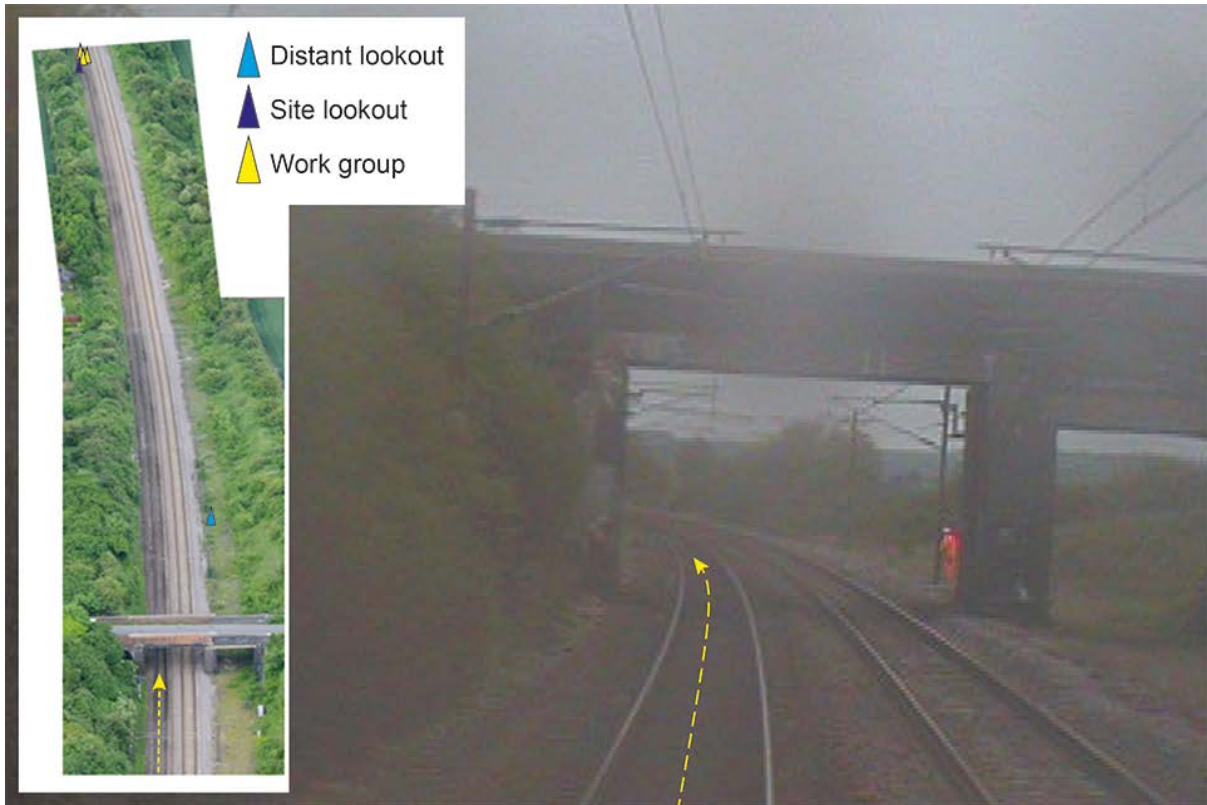
Figure 1: Image from FFCCTV (11:32:53 hrs) from train on the down line. Distant lookout is visible in the up cess (image courtesy of Greater Anglia). The inset image shows aerial view of bridge 1525 and position of the distant lookout.
