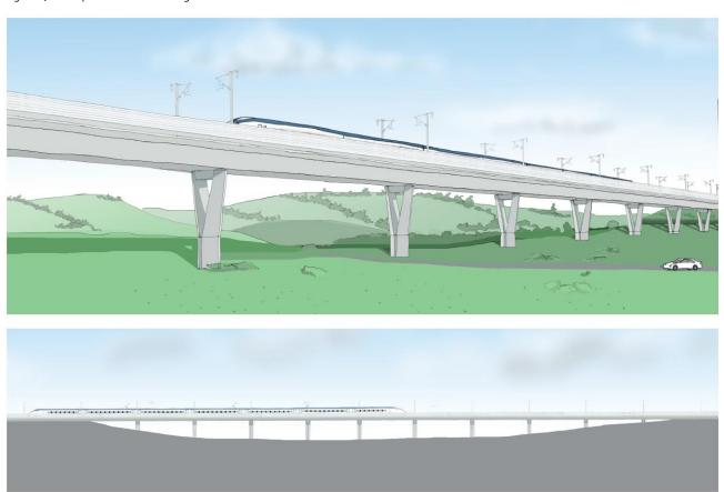
Figure 18: Example illustration of a low viaduct
