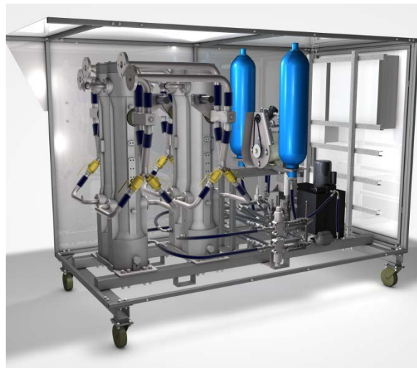
Figure 2.4 Cut-away view of the Exergyn solid state reciprocating engine (Exergyn 2016)
