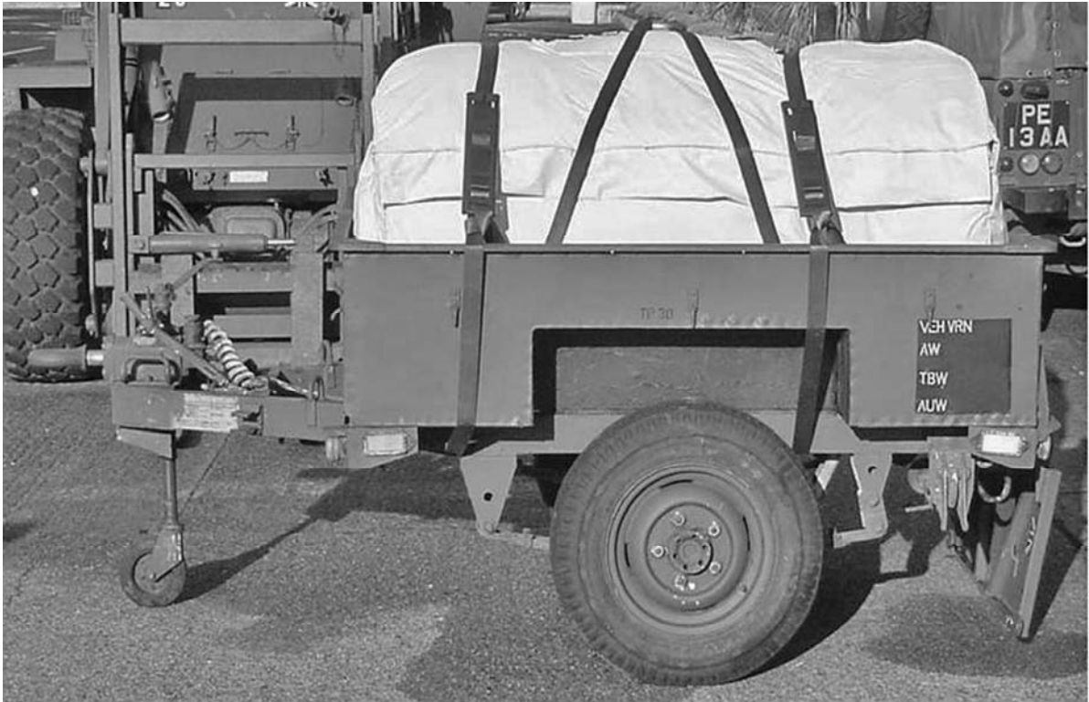
Fig 24 Restraining straps arrangement in the 0.75 tonne GS (wide track) trailer
