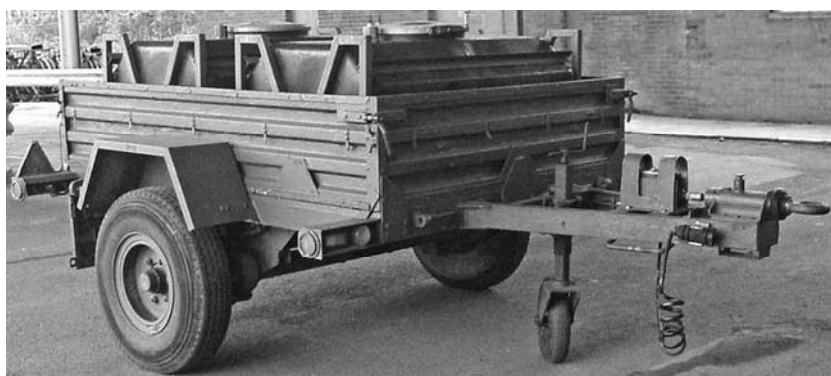
Fig 2 Twin WCP installed in a 1.75 tonne GS trailer - general view
