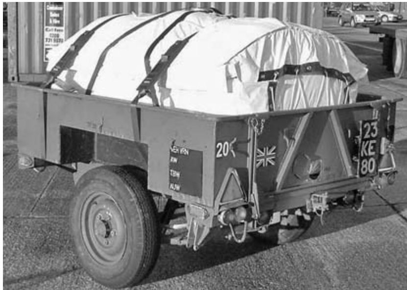
Fig 19 Single insulated water carriage pack installed in the 0.75 tonne GS (wide track) trailer
