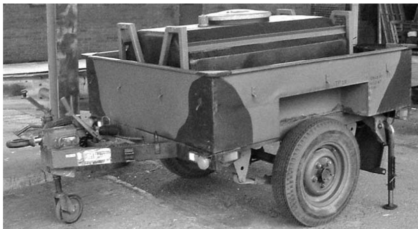
Fig 1 Single WCP installed in a 0.75 tonne GS (wide track) trailer - general view
