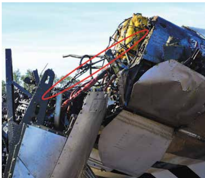
Figure 7 Engine control linkages under tension
