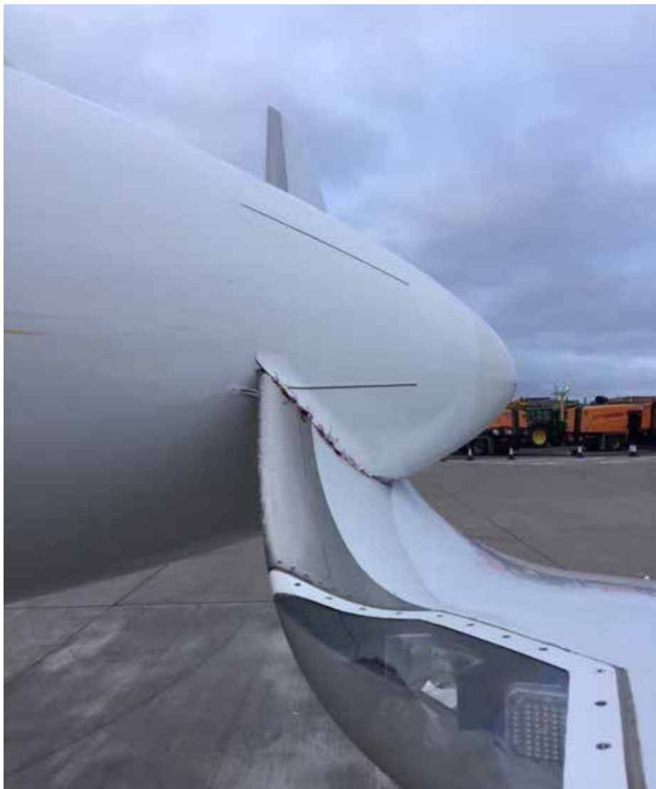
Figure 3 Damage caused by the collision
