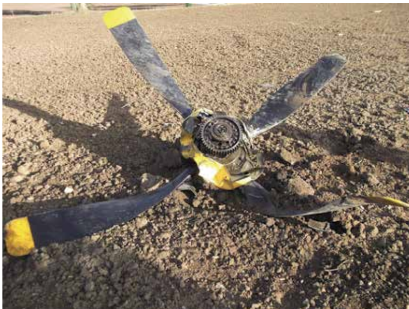
Figure 5 (right) Propeller damage
