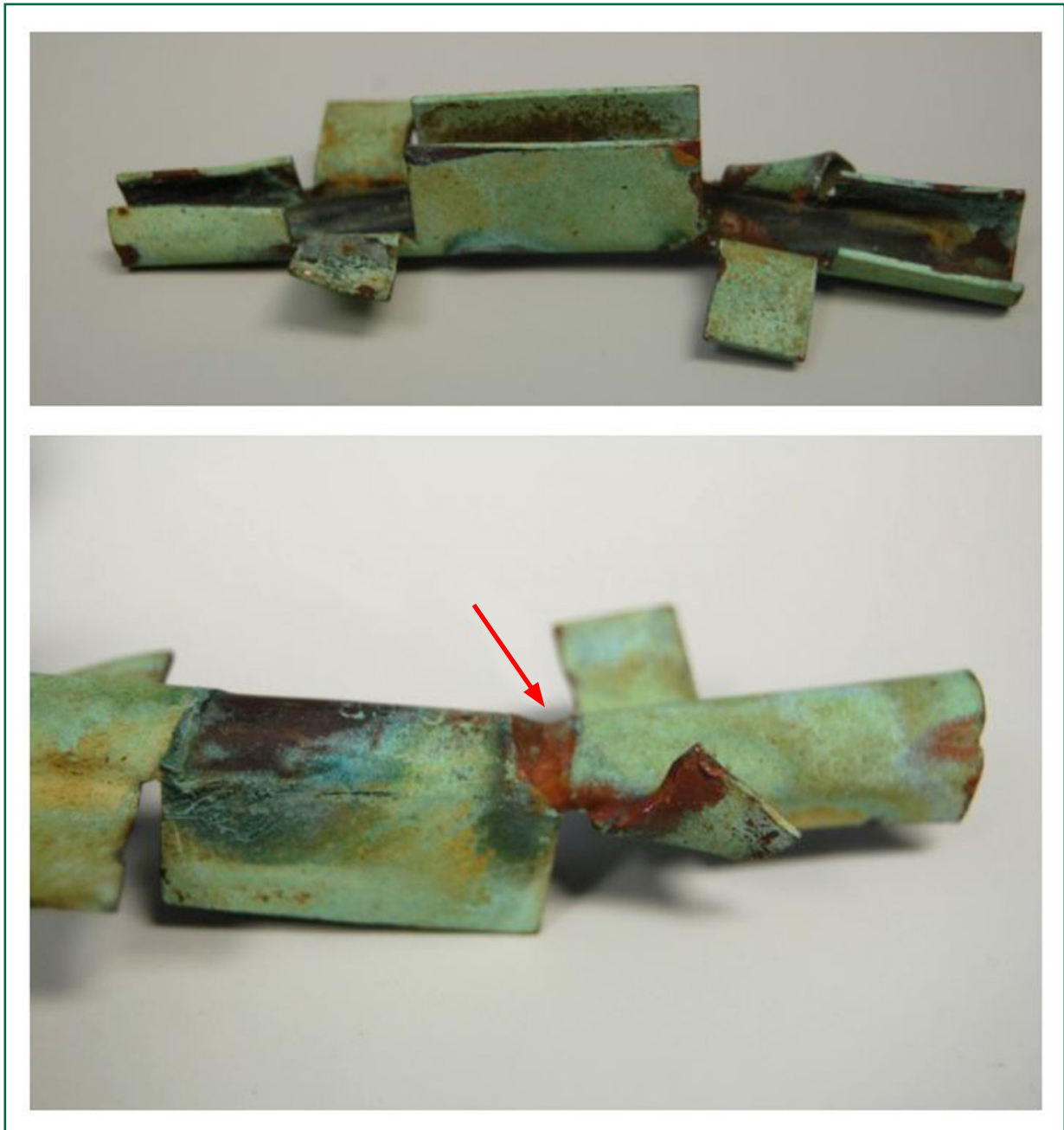
Figure 9: Protective sleeve found at the scene of the accident. Red arrow indicates the groove created from contact with the loop of the auxiliary wire dropper.
