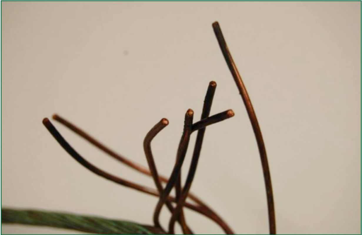
Figure 5: Splayed wire strands on the Liverpool section of the broken auxiliary wire
