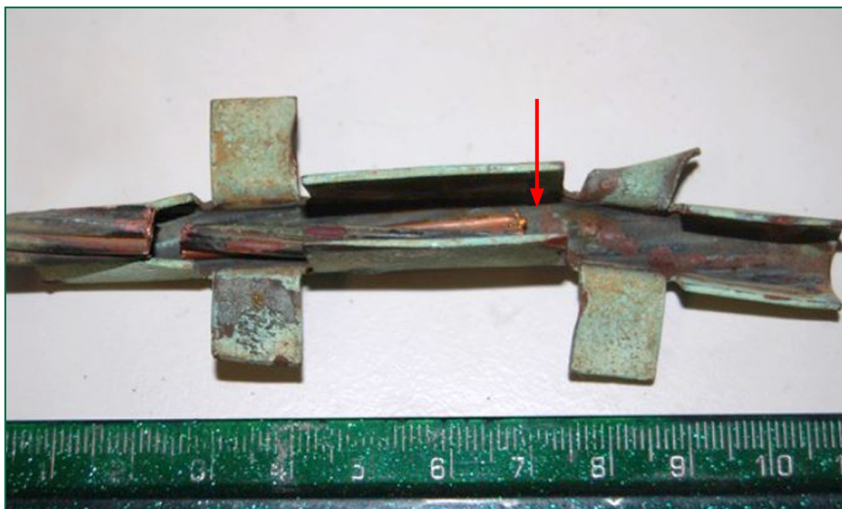
Figure 10: Position of the London end of the broken auxiliary wire relative to the protective sleeve. Red arrow indicates line of wire breakage coincident with the sleeve inner protrusion, which is coincident with the groove shown in figure 9.
