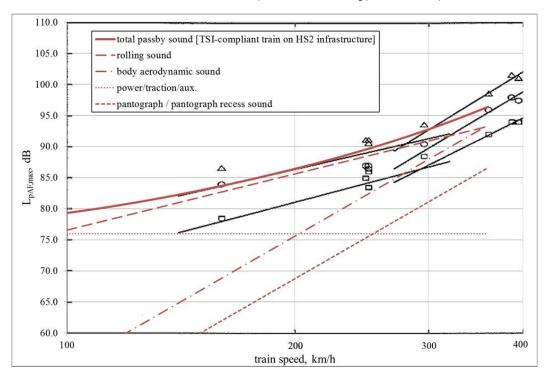
Figure 4:  $L_{pAeq,tp}$  vs speed for total and source component pass-by sound at 25m from the track predicted using the HS2 trains source terms.
