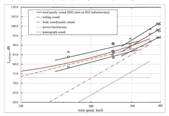
Figure 6:  $L_{pAeq,tp}$  vs speed for total and source component pass-by sound at 25m from the track predicted using the HS2 trains source terms and assuming the train is operating on slab track.
