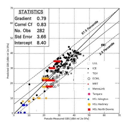
Figure 5 shows the equivalent results for the calculation procedures for perceptible vibration. Again, the monochrome prediction measurement pairs were used to verify the HS1 prediction method. The perceptible vibration data for MRT, Metrolink and Tangara were not available. The prediction measurement pairs for data obtained on the HS1 and predicted with the HS2 method are also shown.
