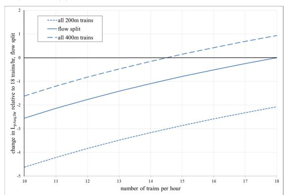
Figure 13: Change in sound level, LpAegrahr, relative to proportion train flow ('flow split' is that assumed in the assessment)
