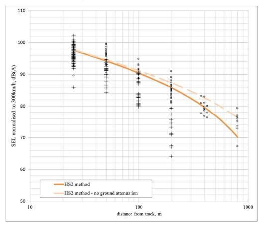
Figure 19: Comparison of HS2 prediction method against measured data,  $L_{pAFmax}$
