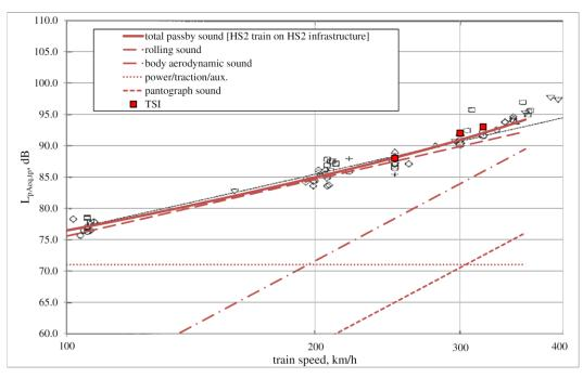
Figure 7:  $L_{pAFmax}$  vs speed for total and source component pass-by sound at 25m from the track predicted using the HS2 trains source terms and assuming the train is operating on slab track.
