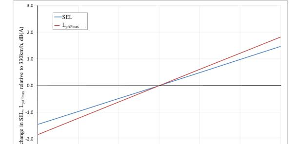
Figure 9: Change in sound level, SEL and L<sub>pAFmax</sub>, relative to train speed
