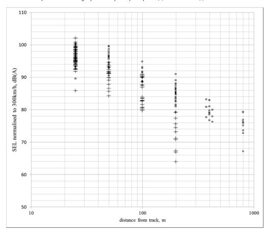
Figure 17: Normalised maximum sound pressure levels of high speed train pass-bys in upwind (+) and downwind (-) measurement conditions.
