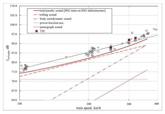
Figure 5: L<sub>pAFmax</sub> vs speed for total and source component pass-by sound at 25m from the track predicted using the HS2 trains source terms.
