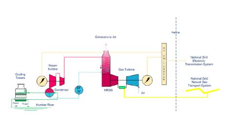
The Main Stack serves the gas turbine and Heat Recovery Steam Generator (HRSG) within the Power island STU. Natural gas will be burnt in the combustion chamber of the gas turbine producing hot, high-pressure gases.
