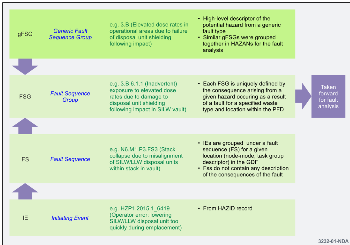
Figure 3 Fault Sequence Development Process
