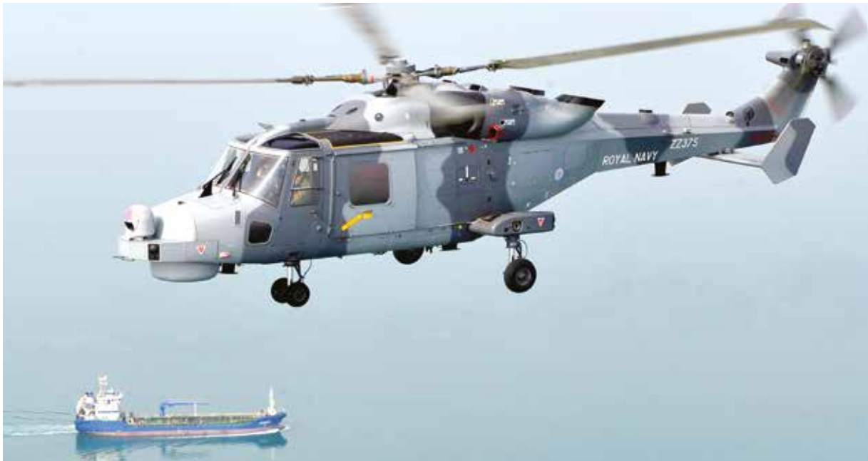
The Royal Navy Wildcat carries out anti-submarine and anti-surface warfare missions in the attack role, as well as missions in the ISR role
