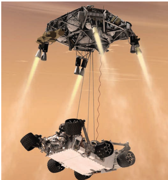
Artist's image showing the sky crane concept being used for the descent of the Curiosity rover
