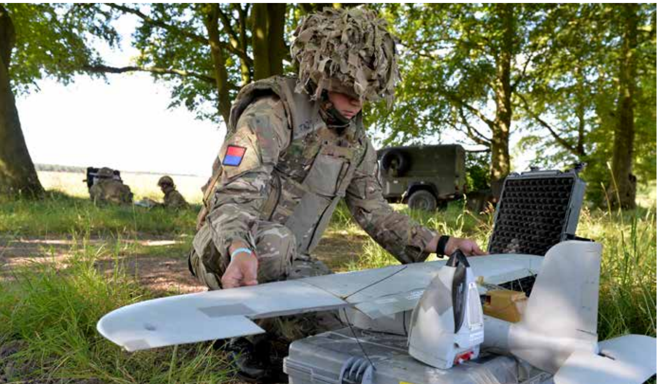
A soldier from the Royal Artillery prepares a Desert Hawk III for flight
