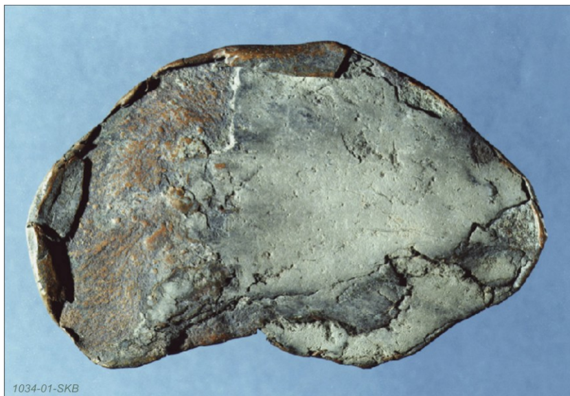
Figure 18 Native copper sample embedded in Devon mudstone (>176 million years old). The sample was found in the Littleham Mudstone formation (Devon, UK). See the Waste Package Evolution Status Report for further discussion of natural analogues of copper behaviour [62, §10.6.2].
