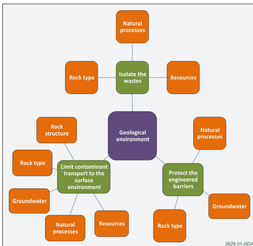
Figure 8 Indication of the types of geological attributes (orange boxes) that determine the different environmental safety functions (green boxes) provided by a geological environment; each attribute shown has sub-attributes as listed in the main text
