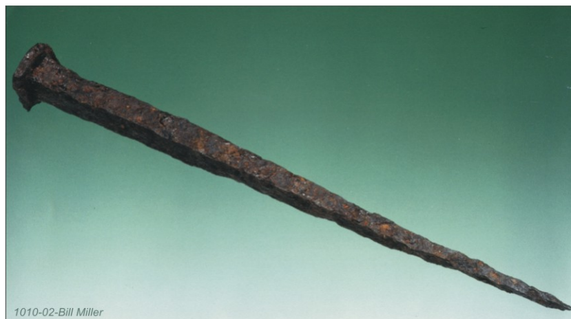
Figure 26 A 30-cm-long Roman nail that had been buried in clay soil in Scotland almost 2,000 years ago [62, §10.7.2]
