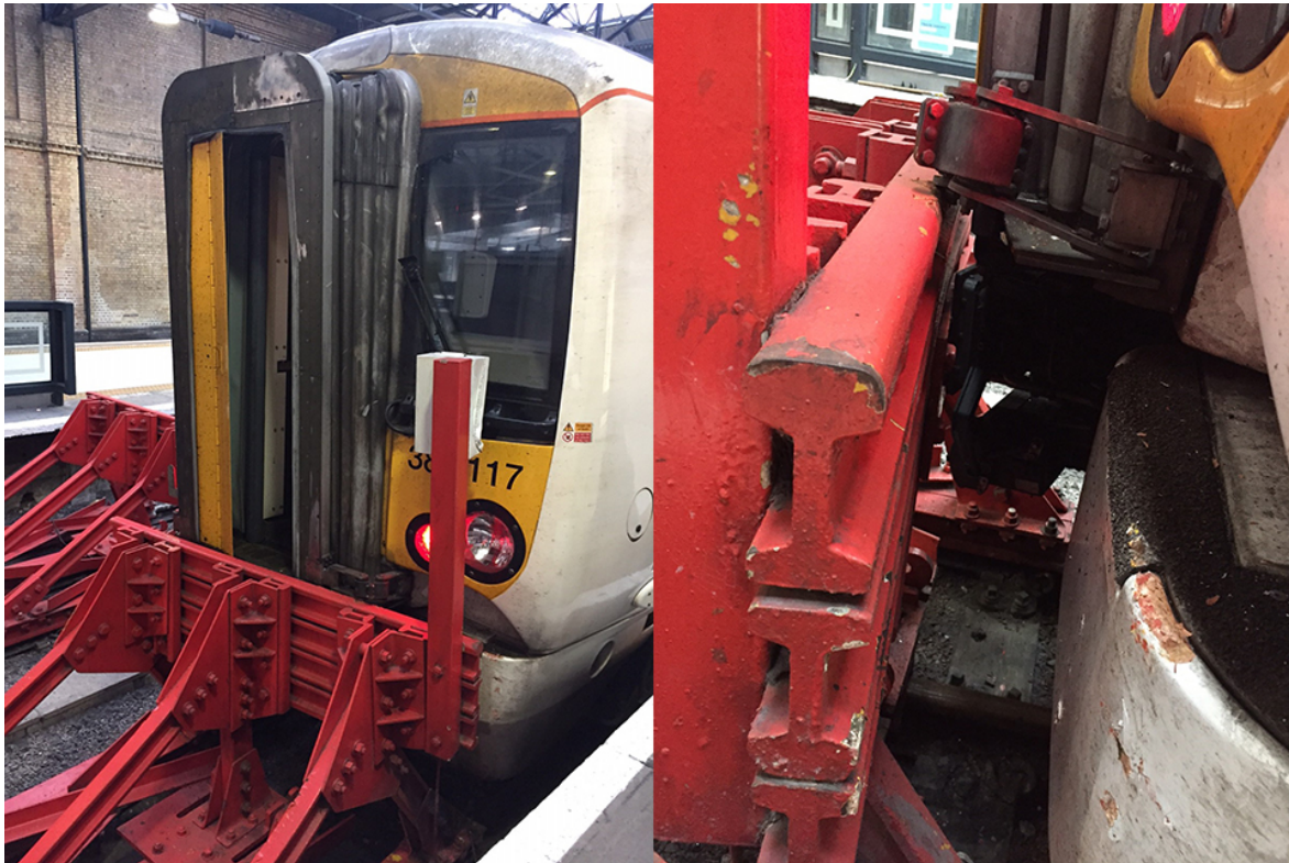
The train and the buffer stops after the collision (images courtesy of Network Rail)
