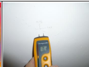
16.8% WME on gable wall RHS of chimney breast
