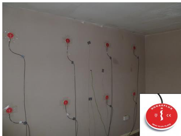
Figure 4: HFP (inset) and HFPs in situ on the control party wall
