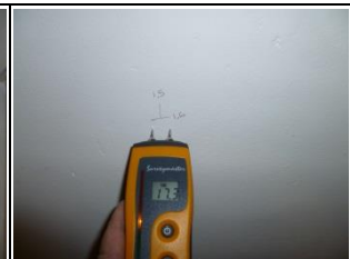
17.8% WME on gable wall LHS of chimney breast
