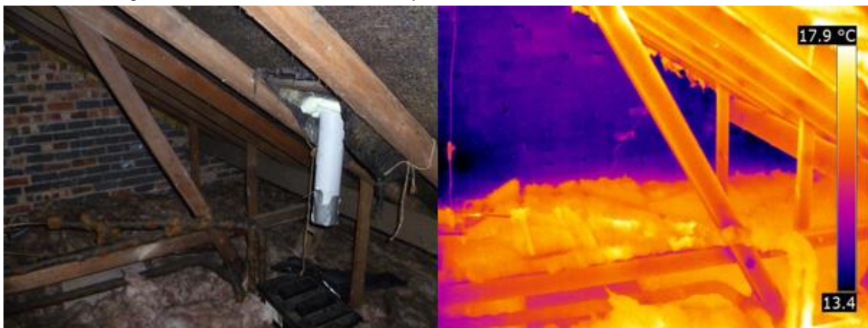
Figure A3: Image and thermogram of the loft space above bedroom 3 with the retrofit loft insulation fitted
