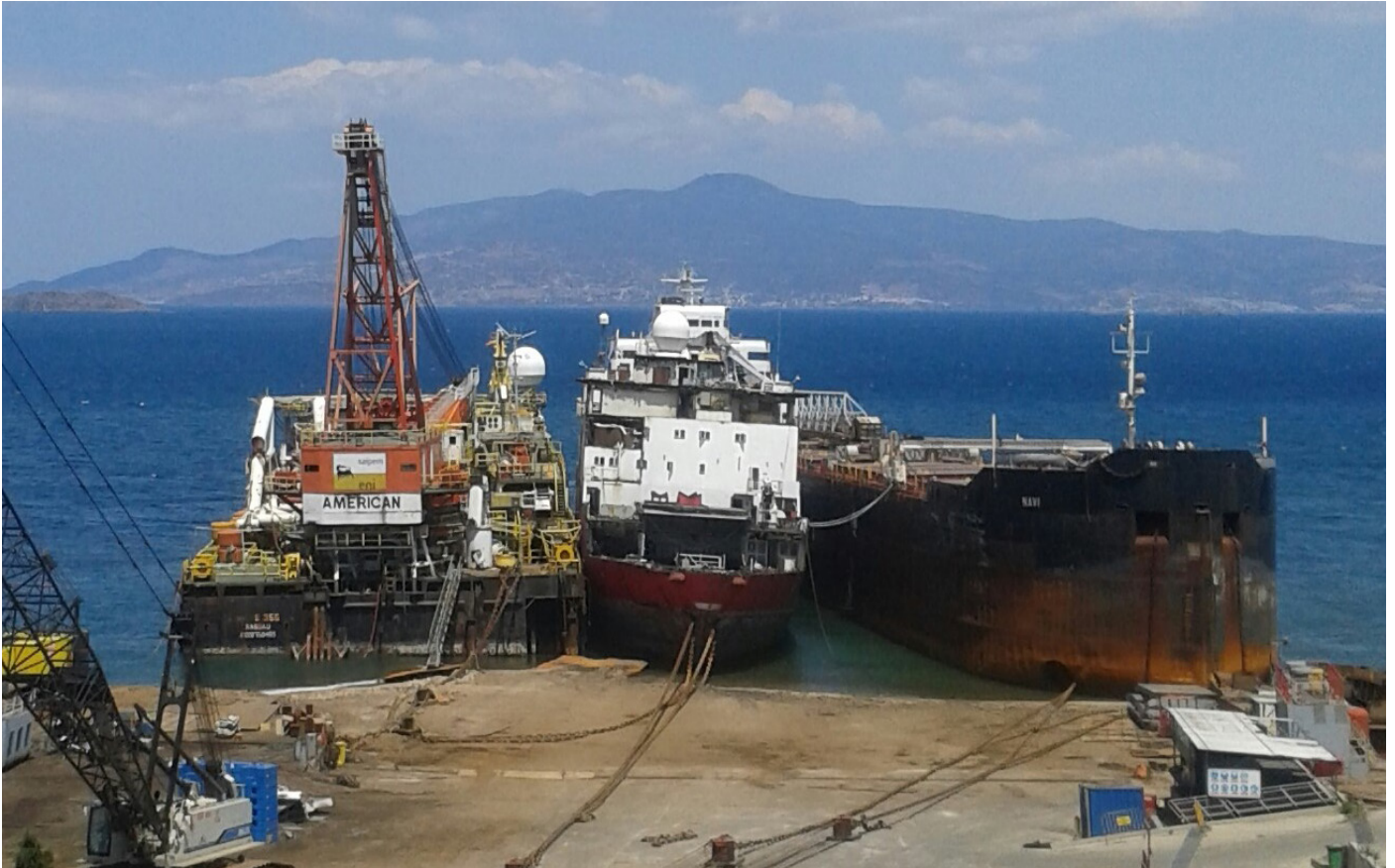
7 July 2016 - showing stages of pre-cutting ready for the hull to be winched up the dry slipway.
