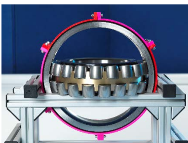
Spherical roller bearing in 3D printed referencing frame used to improve the service lifetime of systems used in wind turbines.
