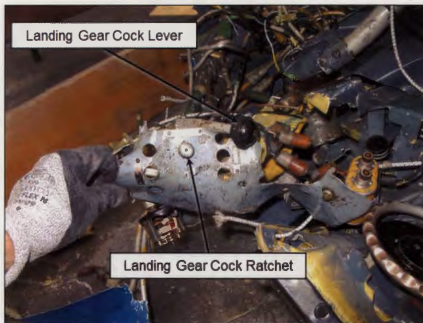
Figure 1.4.15 G-YAKB Front Cockpit Landing Gear Cock Lever in post-accident position. (Source: AAIB.)
