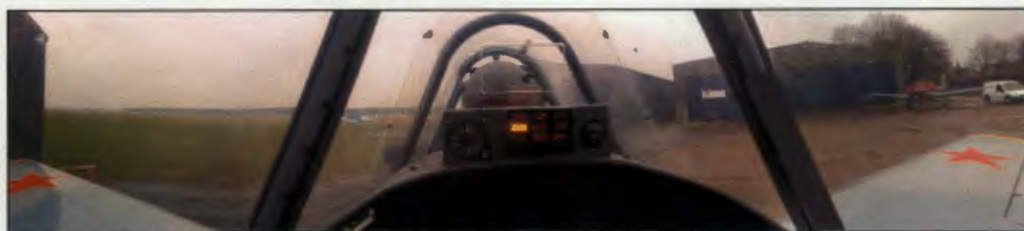
Figure 1.4.5. Yak-52 Rear cockpit Field of View (FOV) forward (180° panoramic). Note with FSP in place forward visibility is reduced, hangar in front obscured and side view obscured by straight wings; the remainder of forward FOV is unaffected.
