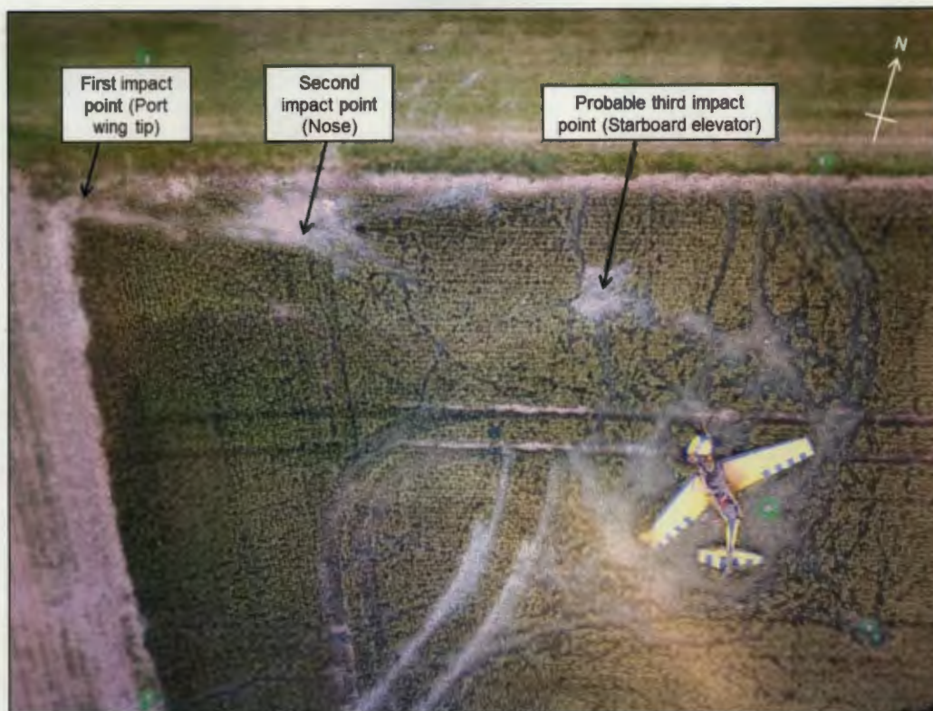
Figure 1.4.12 Aerial View of Crash Site Showing Impact Points
