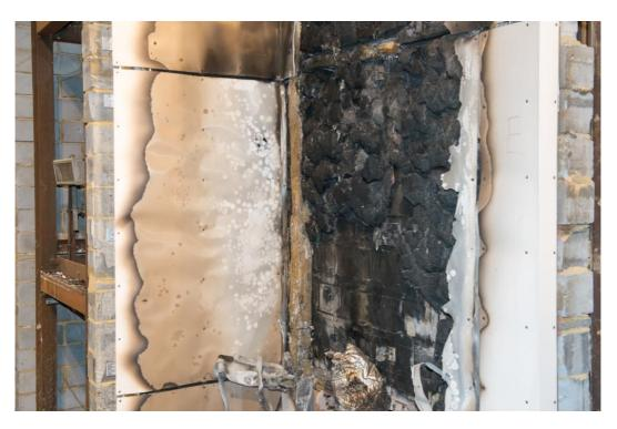
Figure 25. First row ACM panels (directly above combustion chamber).
