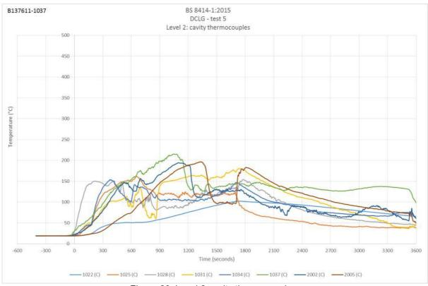
Figure 20. Level 2 cavity thermocouples.
