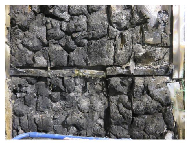
Figure 34. Close up of second cavity barrier in line with the combustion chamber opening.
