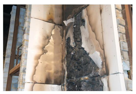
Figure 27. Second row ACM panels (approximately 2300mm-4600mm above combustion chamber).
