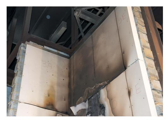
Figure 28. Third row ACM panels (approximately 4600mm-6500mm above combustion chamber).
