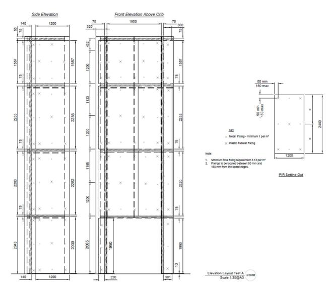
Figure 15. Front elevation, side elevation for the insulation panels installation (supplied by the Test Sponsor).
