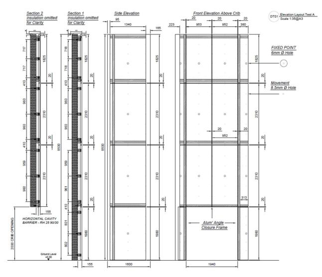
Figure 13. Front elevation, side elevation and vertical sections for the system (supplied by the Test Sponsor)
