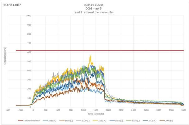
Figure 19. Level 2 external thermocouples.
