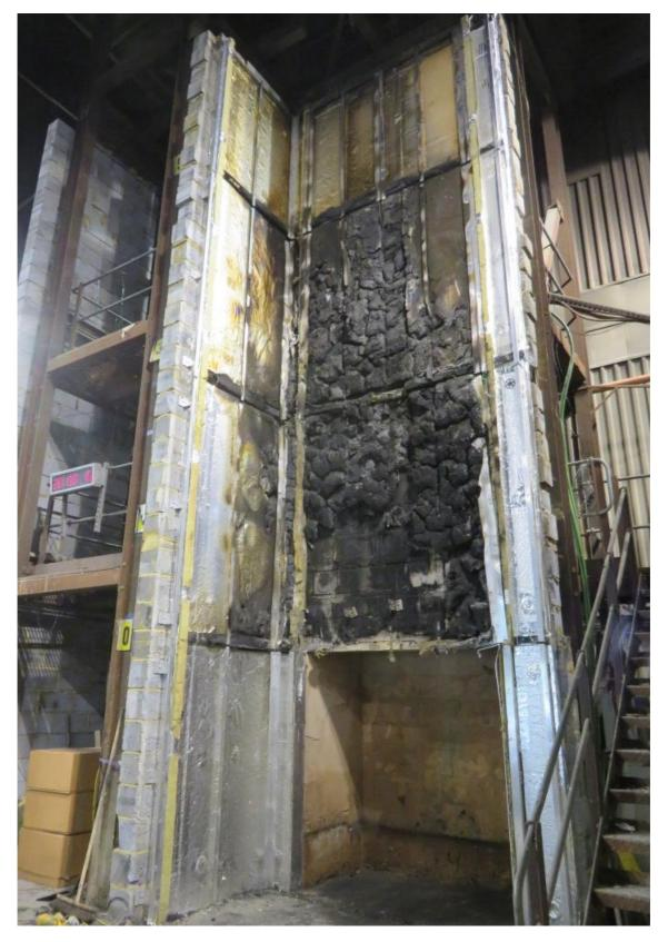
Figure 30. Full height photograph of system following removal of ACM panels.
