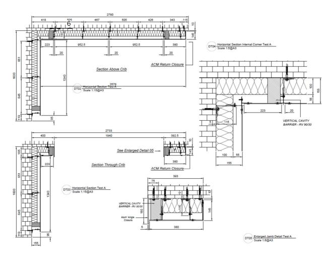
Figure 16. Horizontal section through and above the combustion chamber, and installation details for the system (supplied by the Test Sponsor).
