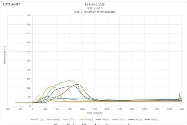
Figure 21. Level 2 insulation thermocouples.
