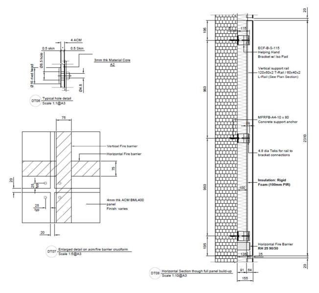
Figure 17. Vertical section through the cladding system, ACM panel detail and vertical and horizontal cavity barriers intersection (supplied by the Test Sponsor).
