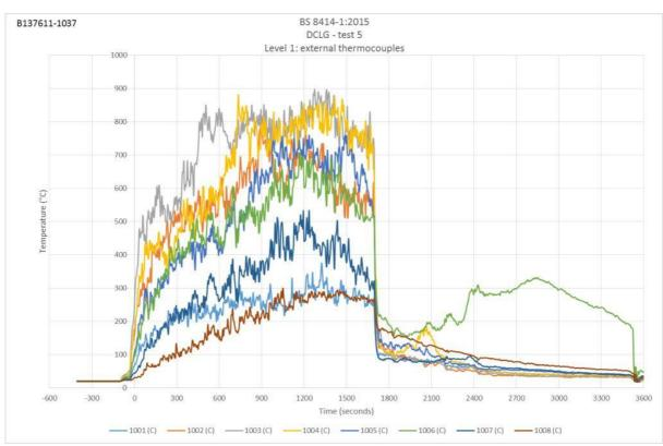
Figure 18. Level 1 external thermocouples.
