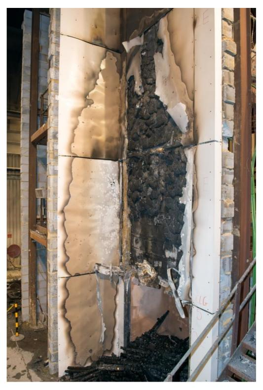
Figure 24. Photograph of system post-test – wing wall.
