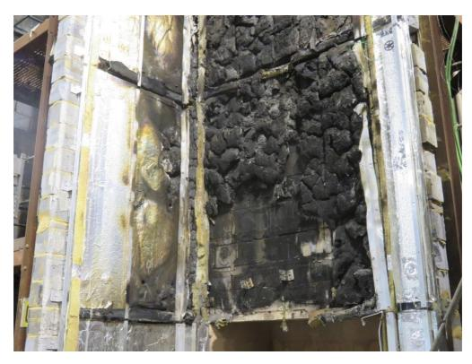
Figure 31. Damage to cladding system beneath ACM panels directly above combustion chamber.
