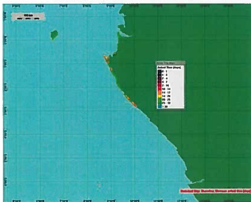
Figure 8-33: Predicted minimum arrival times for oil reaching the shore, derived from stochastic modelling (ENI, 2013).
