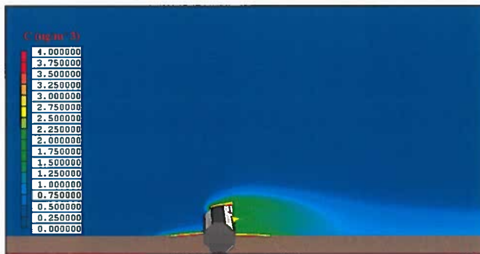
Figure 8-10: Metals concentration around the pipeline ( \mu\text{g}/\text{m}^3 ) – V=0.05 m/s.
