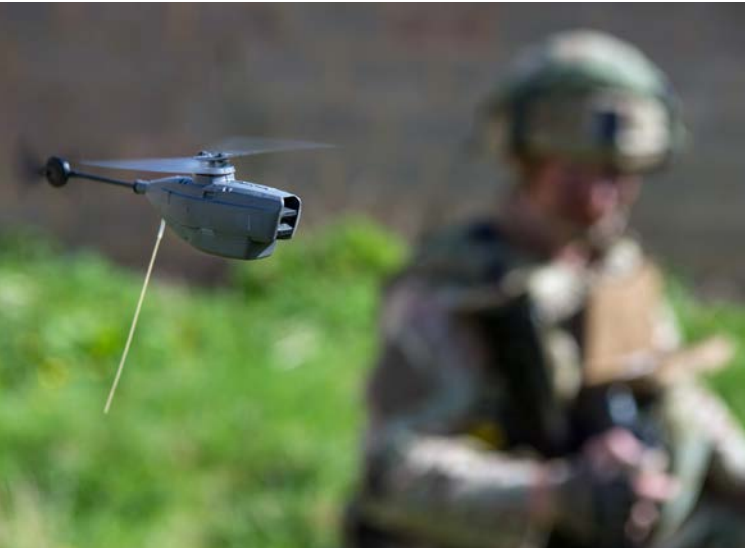
A Black Hornet 2 nano helicopter unmanned aerial vehicle. Crown Copyright.
