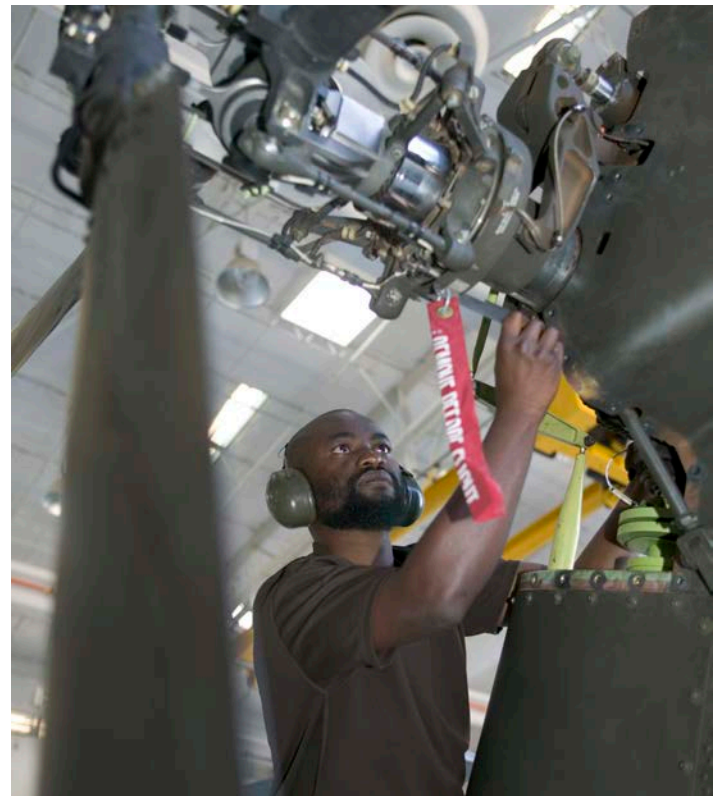
A corporal from the Royal Electrical and Mechanical Engineers inspecting the tail rotor assembly of an Apache during exercise in Arizona, USA. Crown Copyright.
