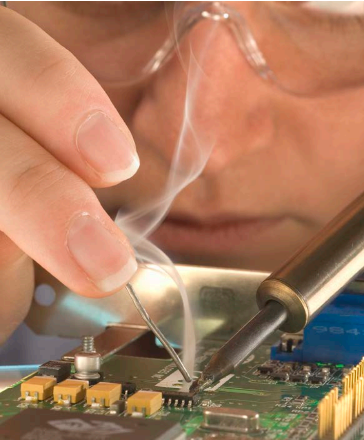
A Royal Air Force Technician solders a circuit board. Crown Copyright.
