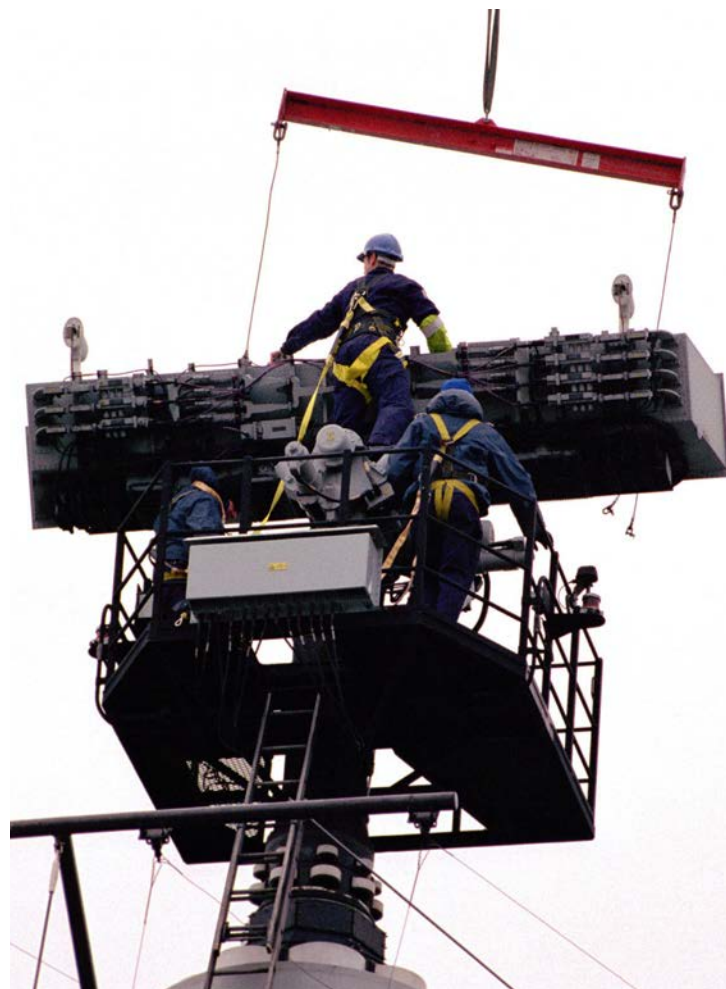
A radar being lifted from the mast of a ship for maintenance. Crown Copyright.
