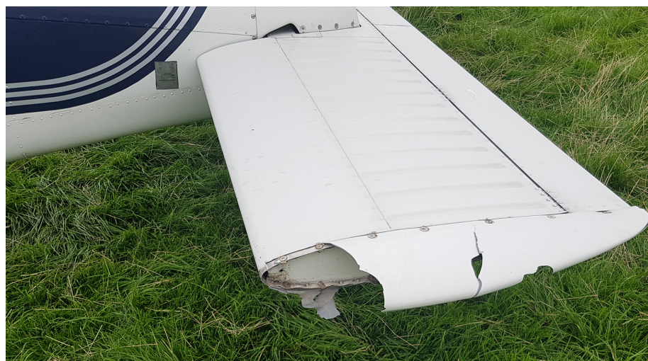
Figure 2 Damage to tip of left stabilator
