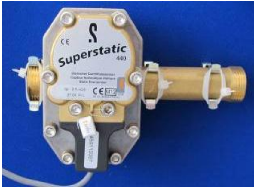
Figure 2-5. Image of Sontex Superstatic 440 heat meter used in the RHPP field trial.
