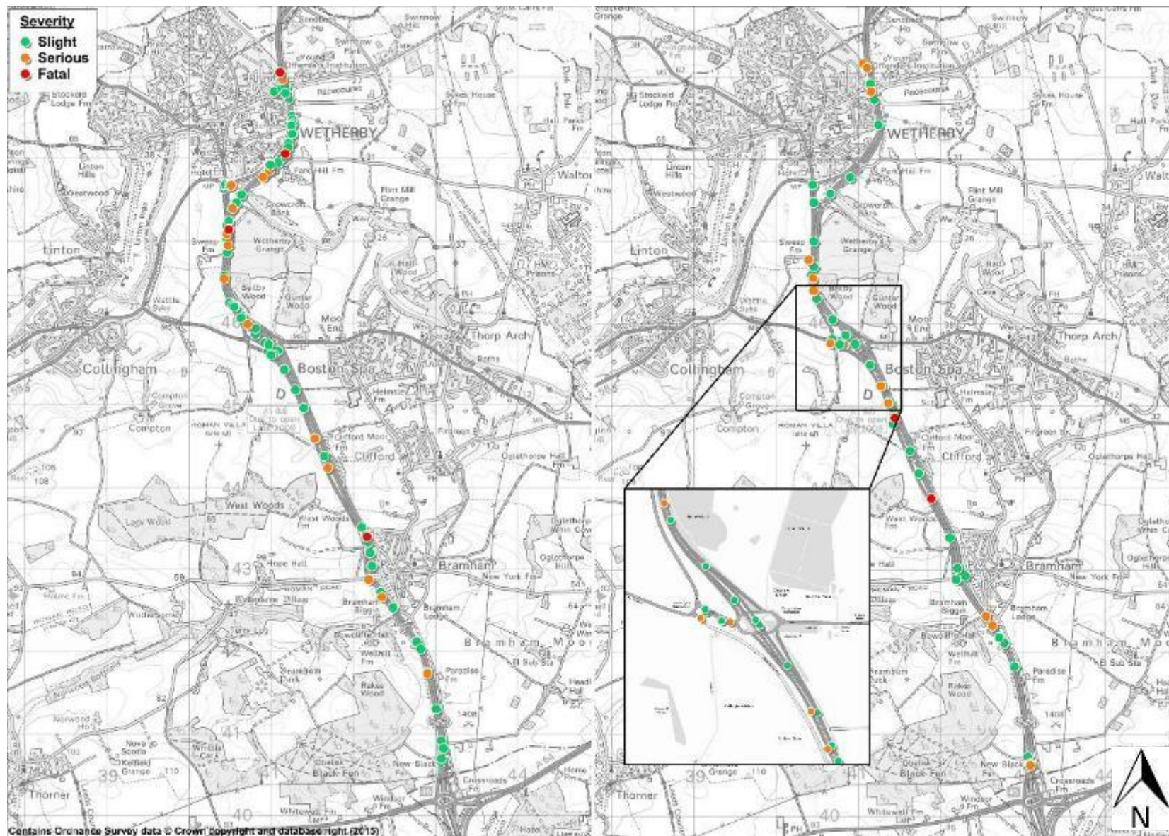
Figure 3.5 Collision Locations on the Key Links: Pre- (Left) and Post- (Right) Scheme Opening
