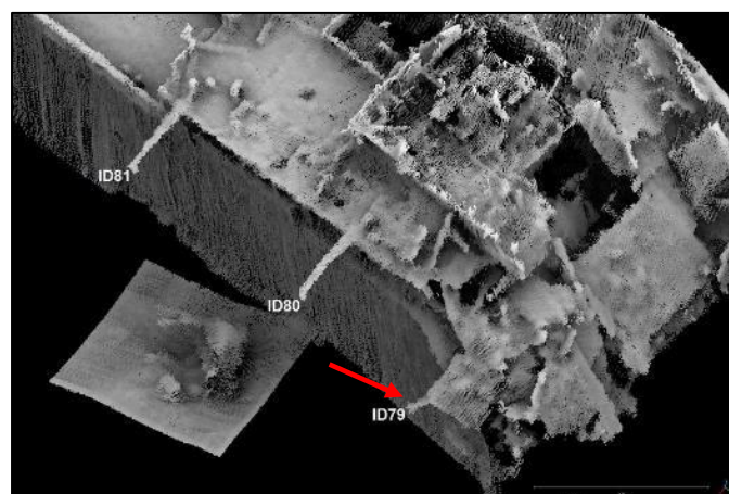
Fig. 20 Lifeboat Davit, starboard side of aft section
