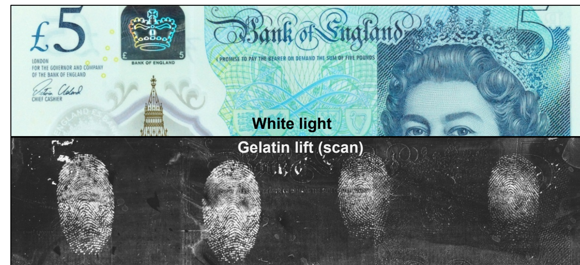
Figure 4: The top half of a £5 banknote treated with titanium dioxide-based powder suspension, when viewed with white light (top) and when imaged from a black gelatin lift (bottom).
