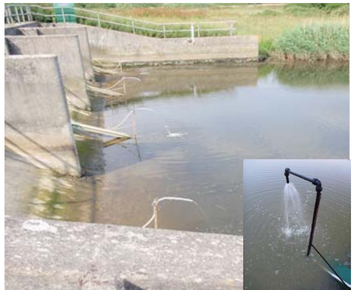
Figure 1: Trials with plunging flow aimed at the base of eel passes which helps young eels find the pass to migrate upstream
