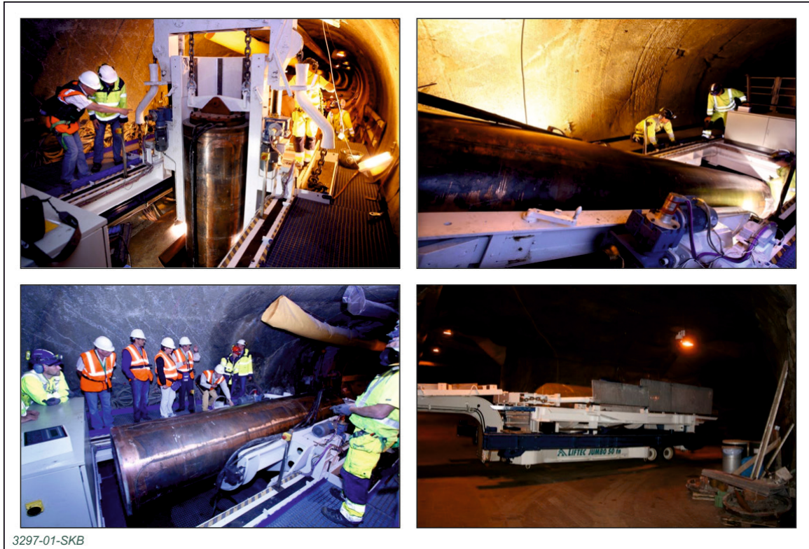
Figure 42: Image from the Prototype Repository project, showing a full scale copper container retrieved after about seven years of emplacement in contact with compacted bentonite in the Aspo URL [443]
