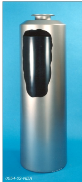
Figure 3: Simulant of vitrified High Level Waste in a stainless steel canister
