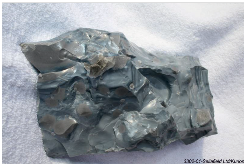
Figure 11: Borosilicate glass incorporating surrogates of Magnox sludge and plutonium-contaminated waste. The glass block is about 15 cm by 10 cm
