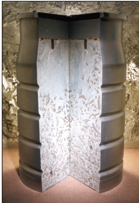
Category 2: In-container grouted wasteform
