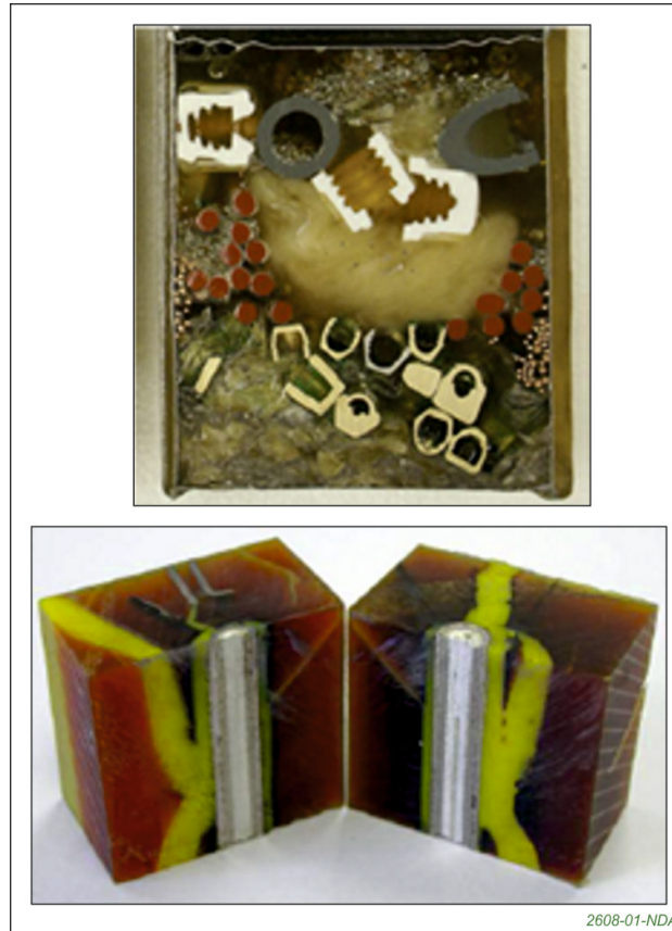
Figure 10: Examples of polymeric encapsulants employed for the immobilisation of some ILW. Top: simulants of radium-contaminated waste encapsulated in VES. Bottom: heating block simulating effect of heat release from graphite (Wigner energy) on encapsulant (epoxy) and ability to infirm any heat-generated crack with further (yellow-coloured) resin
