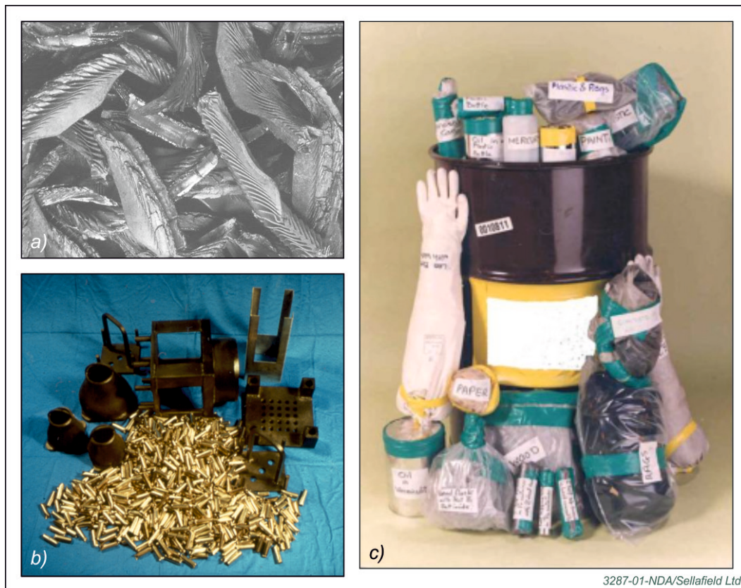
Figure 8: Examples of ILW: a) The cladding of Magnox fuel elements after size reduction (Magnox swarf); b) Parts of PWR fuel elements after size reduction (hulls and ends); c) Plutonium-contaminated materials (PCM)
