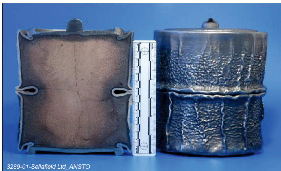
Figure 12: Ceramic from Magnox sludge surrogate (magnesium silicates and titanates), formed by Hot Isostatic Pressing (HIP) – see Box 7. The length of the scale is 15 cm
