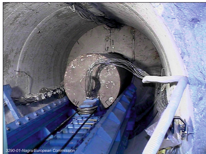
Figure 45: Illustration of the setup of the Materials Corrosion Test (MaCoTe)
