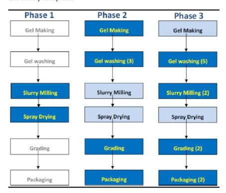
The plant will be housed in the shell of an existing building, on a parcel of land that will be brought into the installation site boundary. The ES2 process is identical to the existing ES1 process, with the gel making, washing and slurry milling taking place on the 'wet side' and the spray drying, grading and packaging taking place on the 'dry side'.
