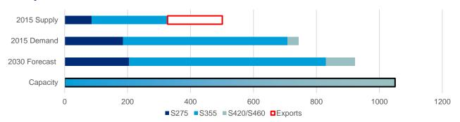
Like the medium section mill, the beam mill lacks thermomechanical rolling facilities, which prevents it supplying products for this higher-value 5% of the market.
