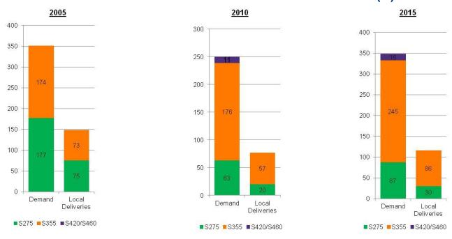
\$420/\$460 are usually M grades – thermo mechanically rolled
