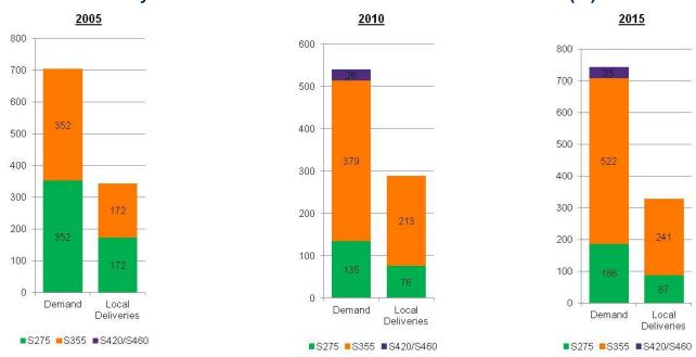
S420/S460 are usually M grades - thermo mechanically rolled
