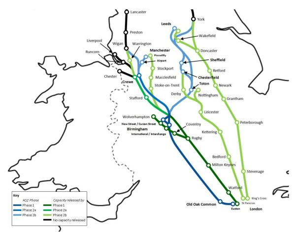
Figure 4 Existing rail lines where capacity for new services is made available by each phase of HS2
