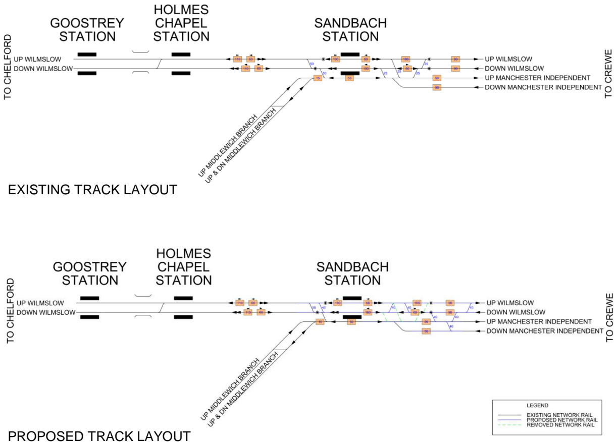
Figure 4: Schematic diagram of existing and proposed track layout at Sandbach Station
