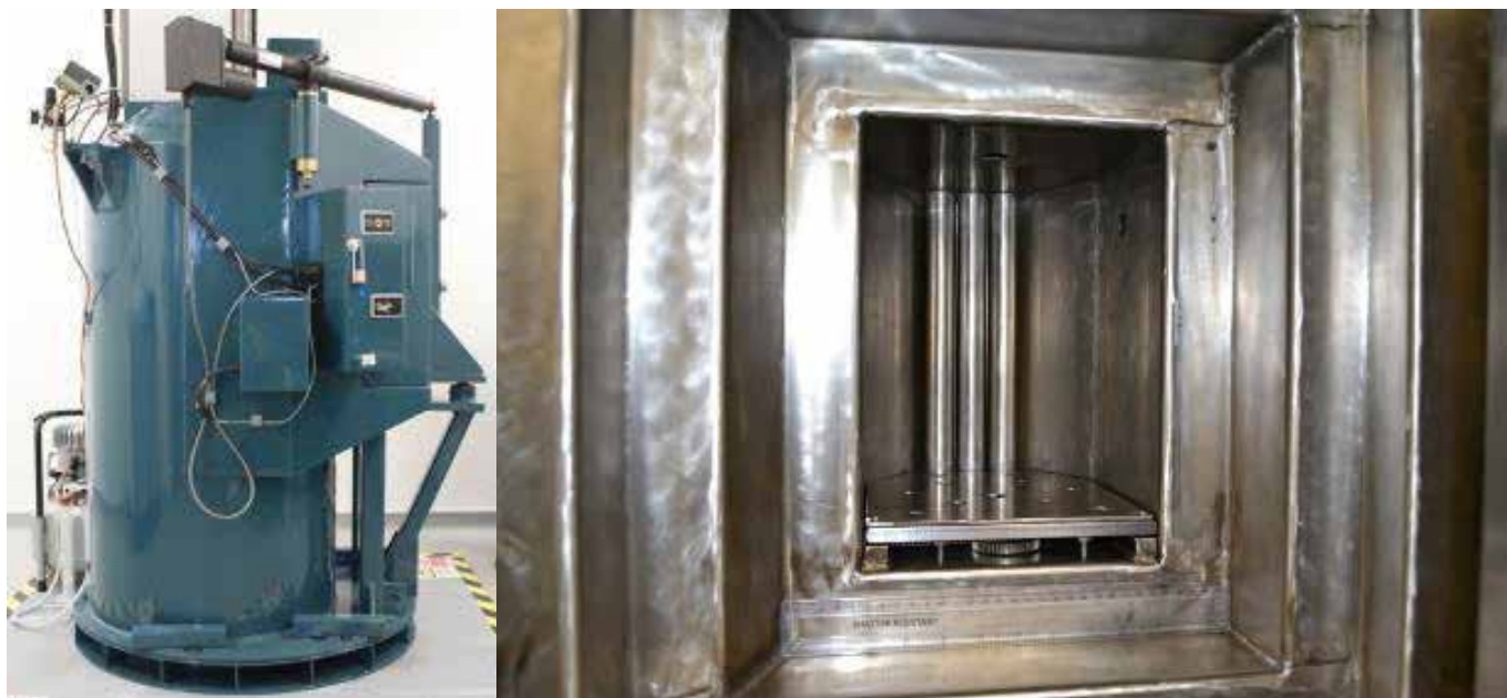
Co60 gamma irradiator and inner chamber (Dalton Cumbrian Facility)
