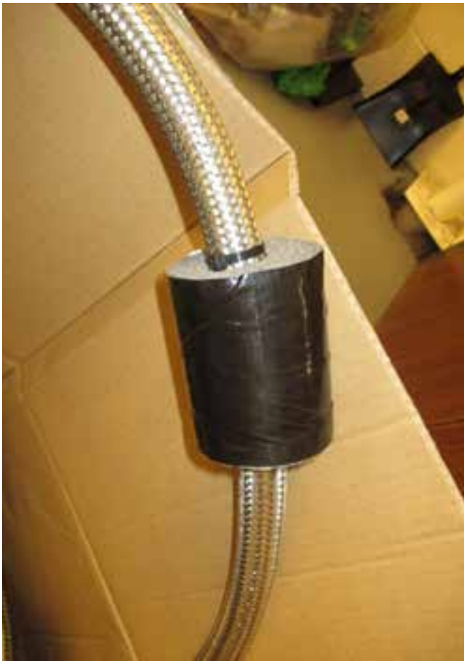
Close up of hose with buoyancy aid
