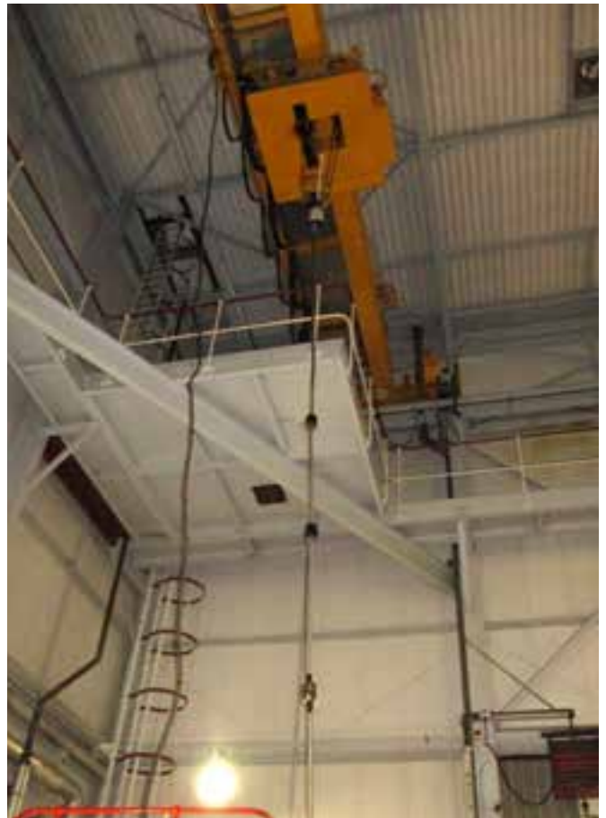
View of stainless steel hose and float system taken during high level flow testing
