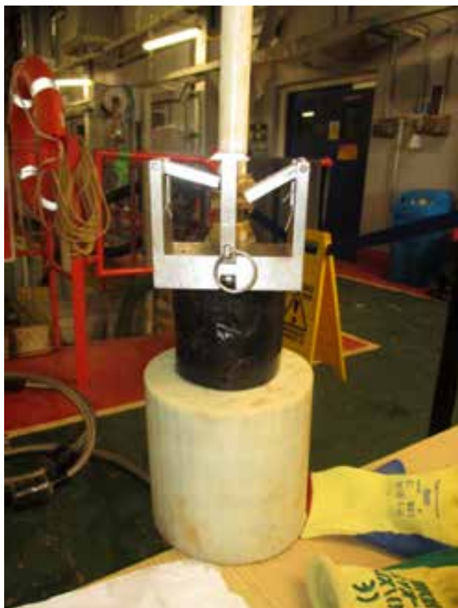
Prototype outlet spout front view with aluminium latching mechanism and cylindrical floats to improve buoyancy for ROV installation
