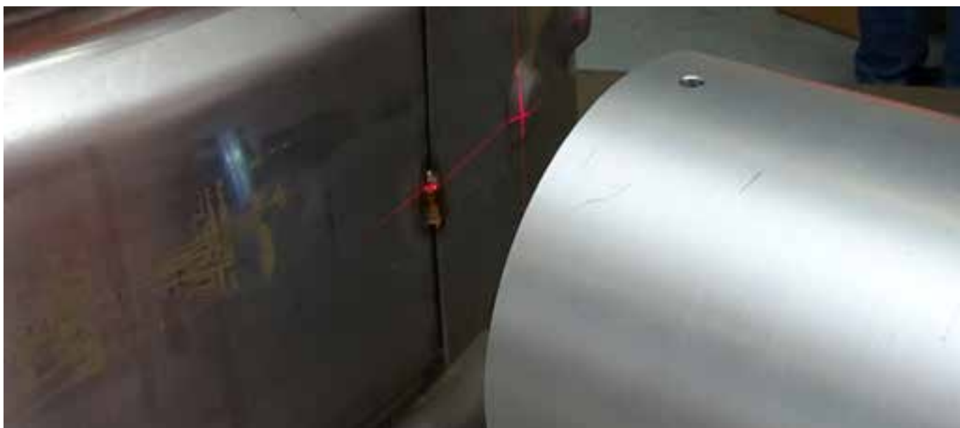
Laser cross hairs highlighting surface defects
