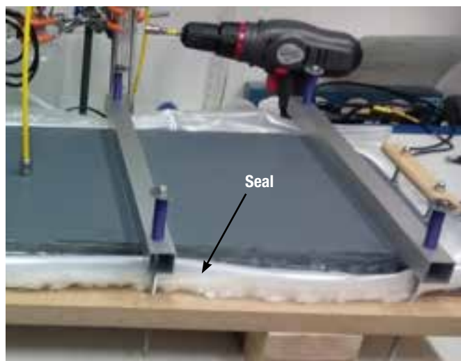
Medium scale assembly for measuring leakage through the seal being tested
