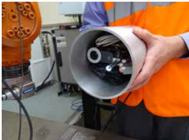
Optical camera system - components in enclosure
