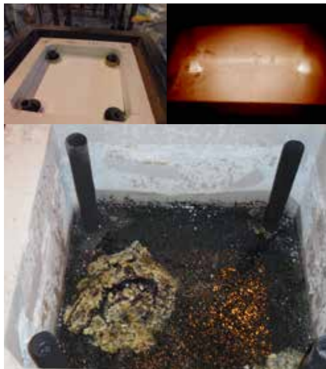
Magnesium hydroxide sludge demonstration (before, during, after)
