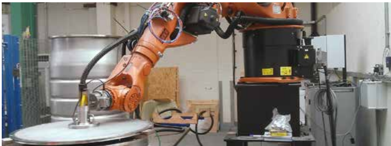
Mass spectrometer trial - sampling through vent on 500L drum
