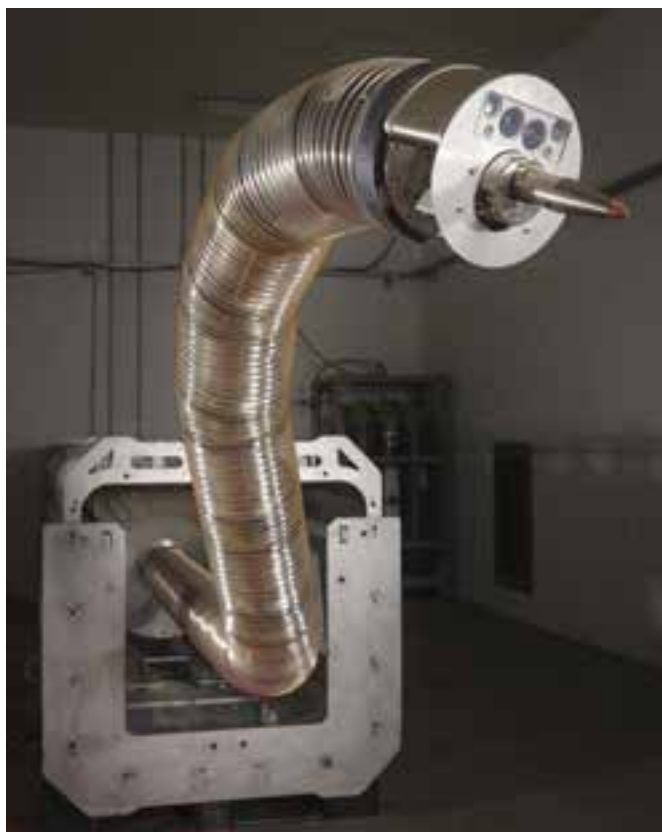
LaserSnake within its housing
