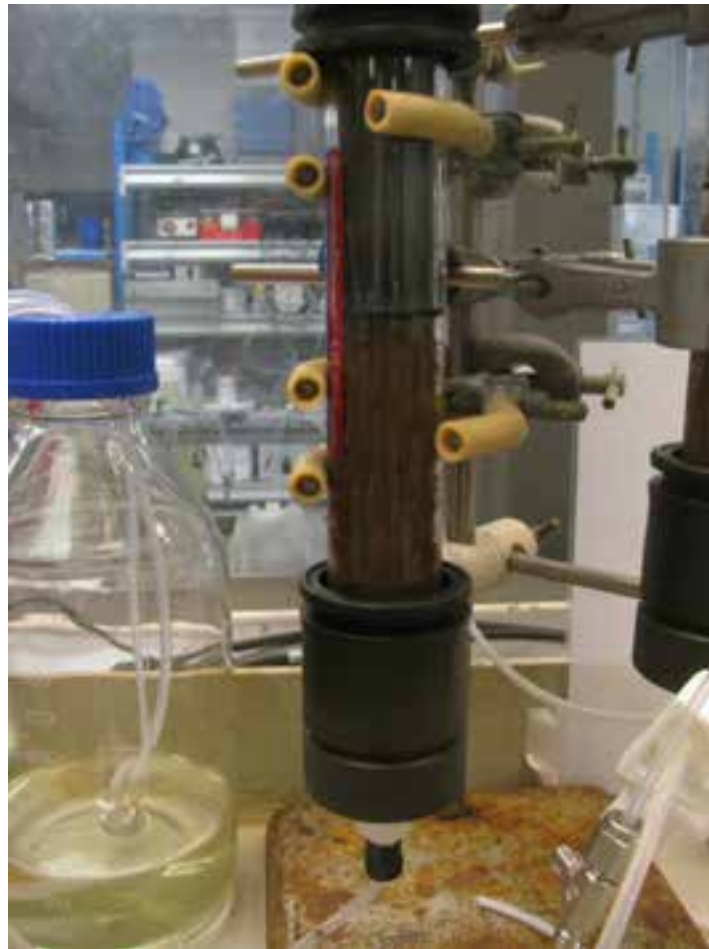
Column testing of reagents in NNL facilities, to assess performance with Sellafield soils and potential groundwater contaminants
