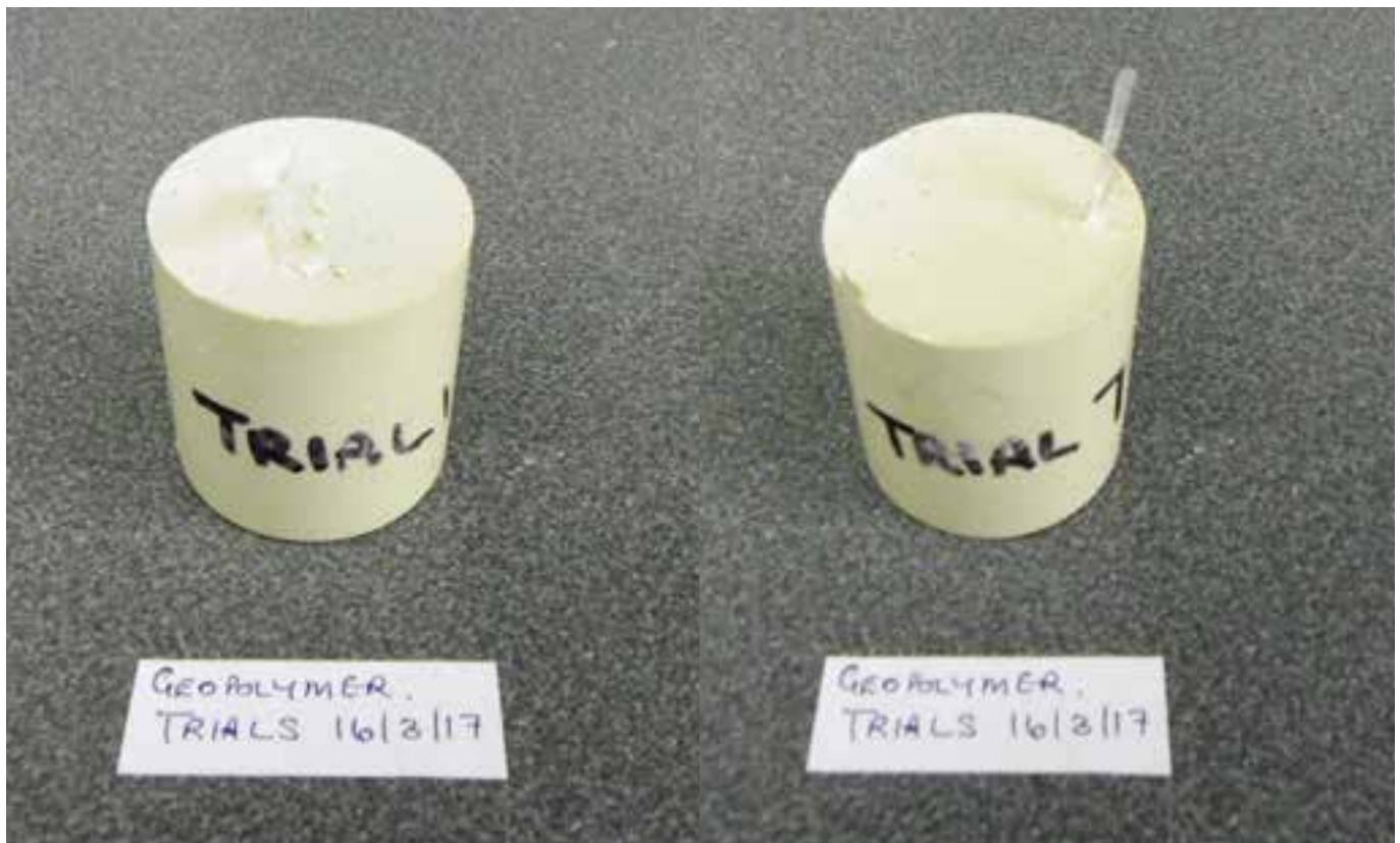
The images are from small scale geopolymer trials completed in March 2017. 2017/18 will see the scaling up of this work to produce products for longer term product quality testing such as strength and dimensional stability.
