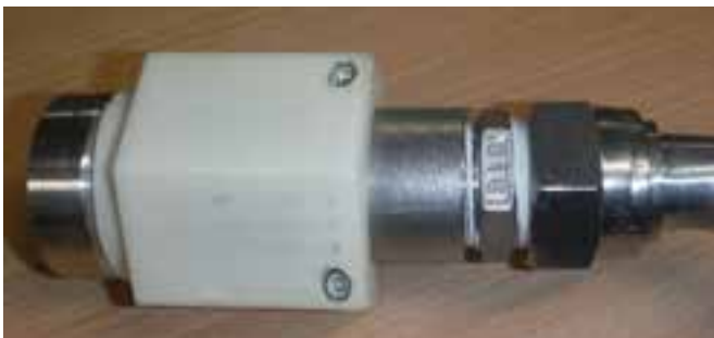
3D printed connector (white part) developed during design trials
