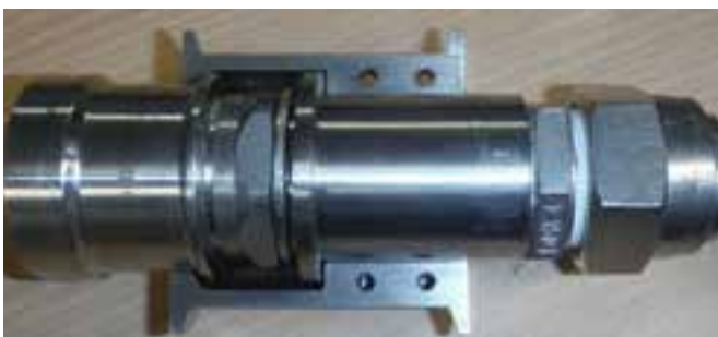
Machined connector based on the final design from the 3D printing trials
