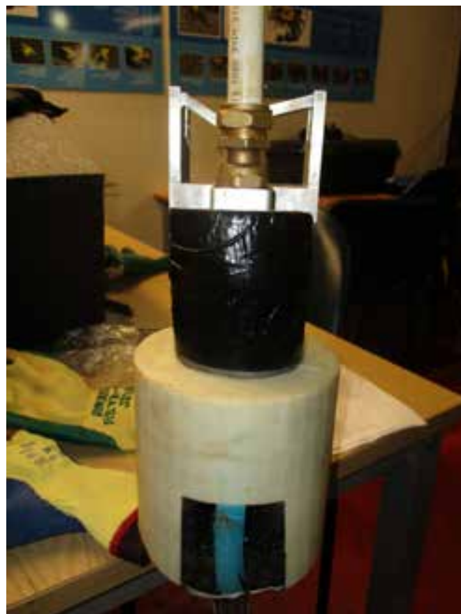
Prototype outlet spout rear view with ROV grip on cylindrical float
