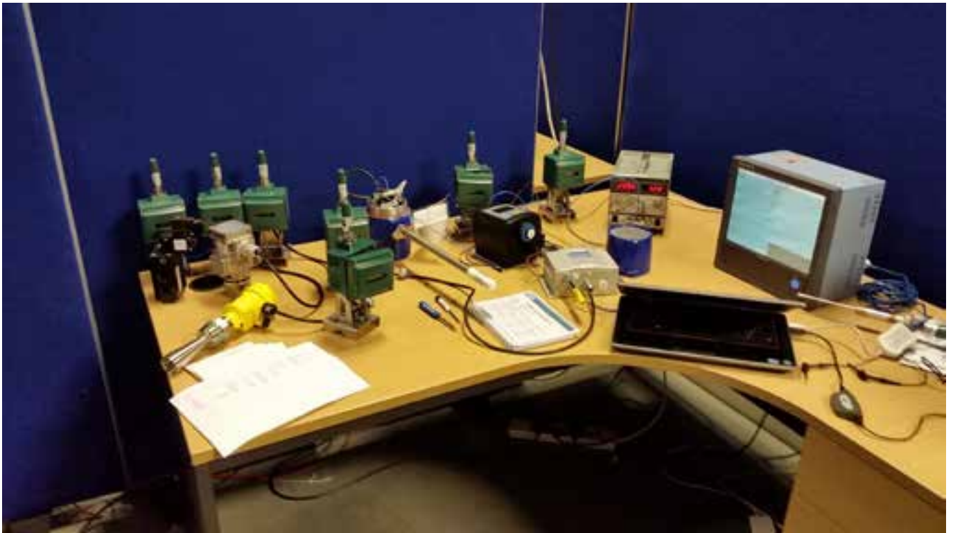
Some of the wired instruments adapted to ISA100Wireless®
