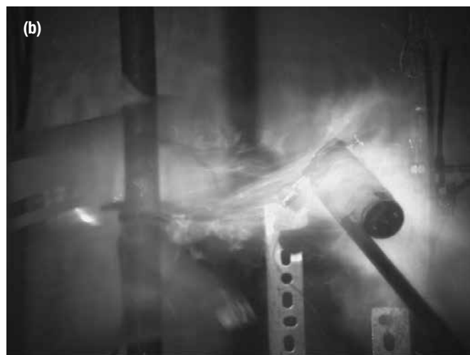
Images illustrating the explosion following the ignition of a small volume of hydrogen in a plastic bag: (a) the ignition source is positioned next to the plastic bag containing hydrogen; (b) the hydrogen mixture in the bag is ignited resulting in an explosion
