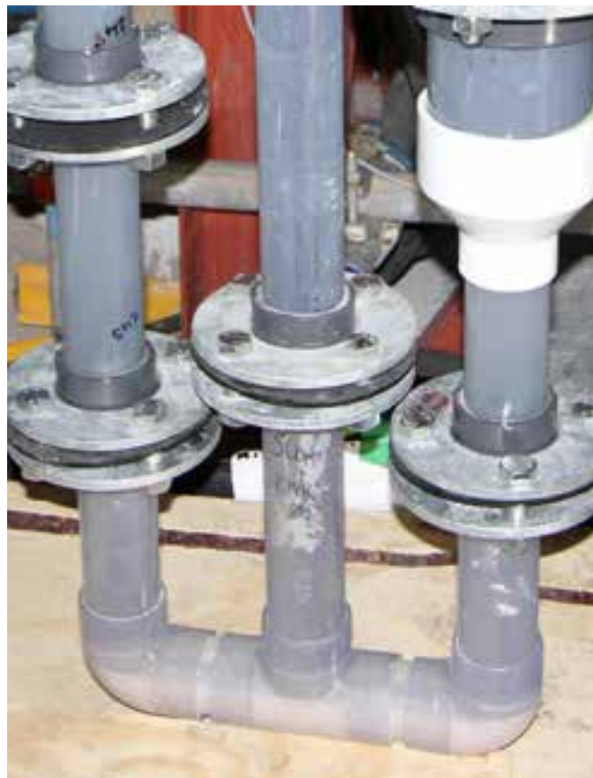
The image shows the solid simulants in the lute feed of the Lute Test Rig
