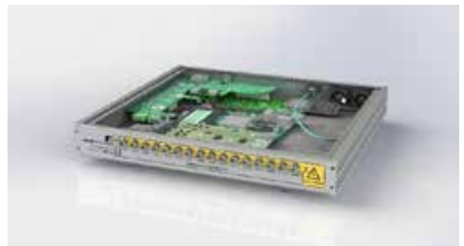
Acoustic backscatter commercialised unit (courtesy of the University of Leeds)
