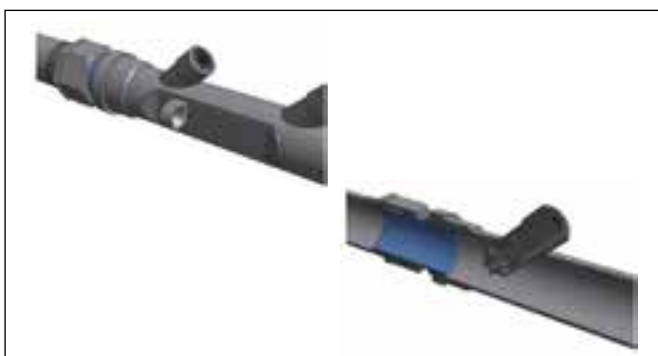
Acoustic backscatter transducer deployment array - transducer mounts developed by James Fisher Nuclear Ltd.
